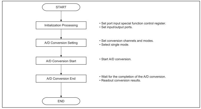
Figure 4.2.1 Basic Process Flow for the A/D Converter
