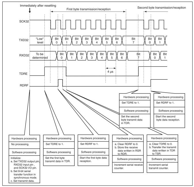
Figure 3.1 Operation Principle of Simultaneous Serial Data Transmission/Reception in Synchronous Mode
