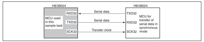
Figure 1.1 Simultaneous Serial Data Transmission/Reception in Synchronous Mode
