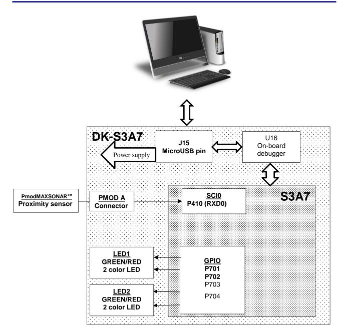
Figure 1 Block diagram
