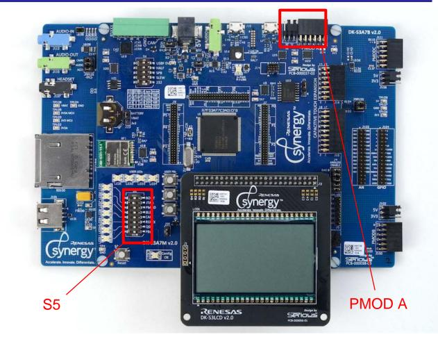
Figure 2 External view of the DK-S3A7
