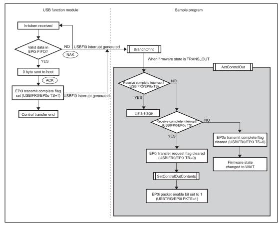
Figure 5.10 Status Stage (Control-Out Transfer)
