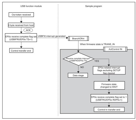
Figure 5.9 Status Stage (Control-In Transfer)
