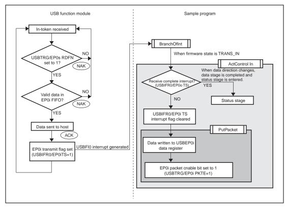
Figure 5.7 Data Stage (Control-In Transfer)
