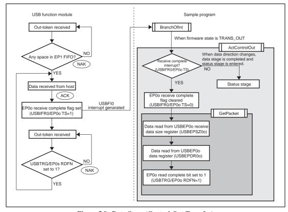
Figure 5.8 Data Stage (Control-Out Transfer)
