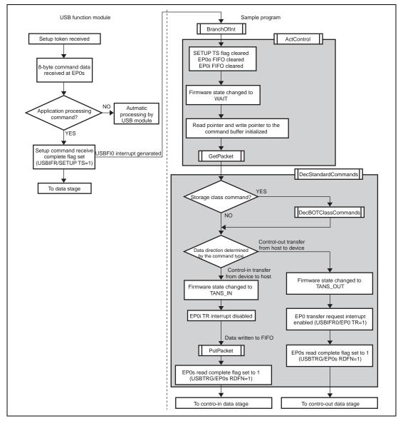
Figure 5.6 Setup Stage
