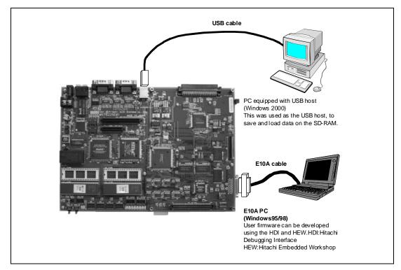
Figure 3.1 Device Connections
