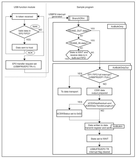
Figure 5.17 Status Transport (Data Transport Bulk-Out Transport)
