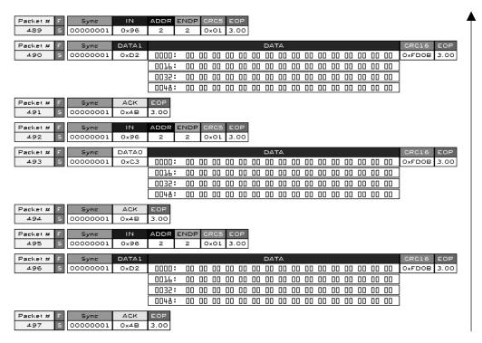
Packet # F Sync IN ADDR ENDP CRC5 EOP 498 \$ 00000001 0x96 2 2 0x01 3.00 DATA (data transport)
