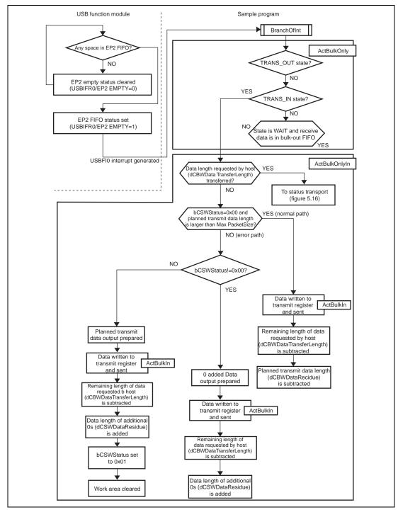
Figure 5.14 Data Trans port (Bulk-In Transport)
