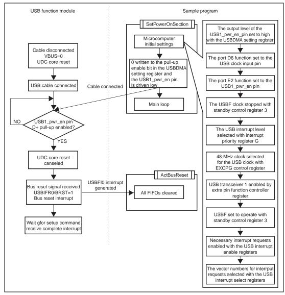
Figure 5.3 Interrupt on Cable Connection
