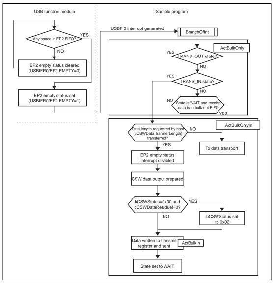
Figure 5.16 Status Transport (Data Transport Bulk-In Transport)
