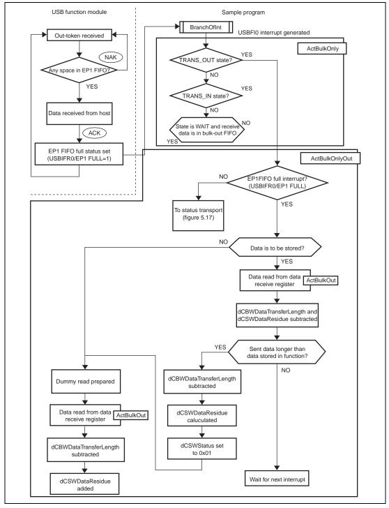
Figure 5.15 Data Transport (Bulk-Out Transport)
