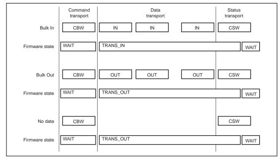
Figure 5.12 Various Stages in Bulk-Only Transport
