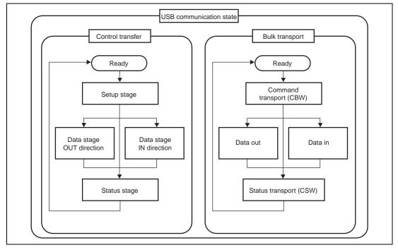
Figure 4.2 USB Communication State
