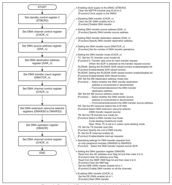
Figure 2 Example of Flow for Initialization of the DMAC
