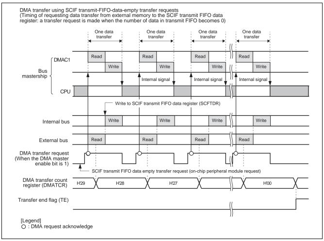
Figure 3 Operation Timing of Sample Application
