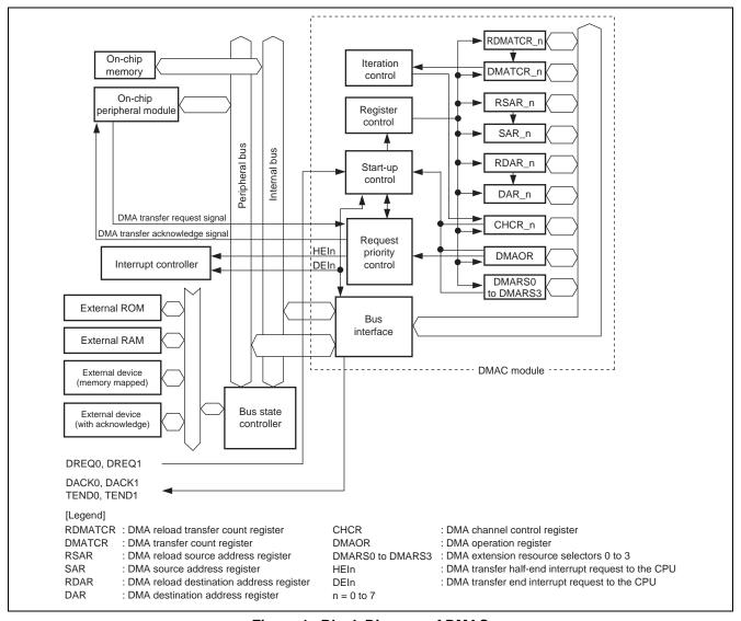
Figure 1 Block Diagram of DMAC
