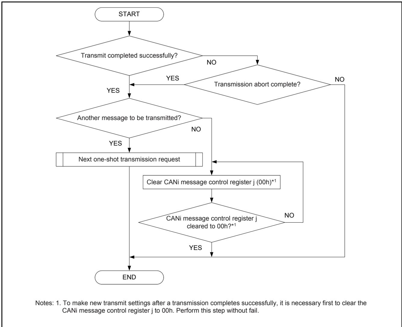
Figure 10 One-Shot Transmission Complete Procedure
