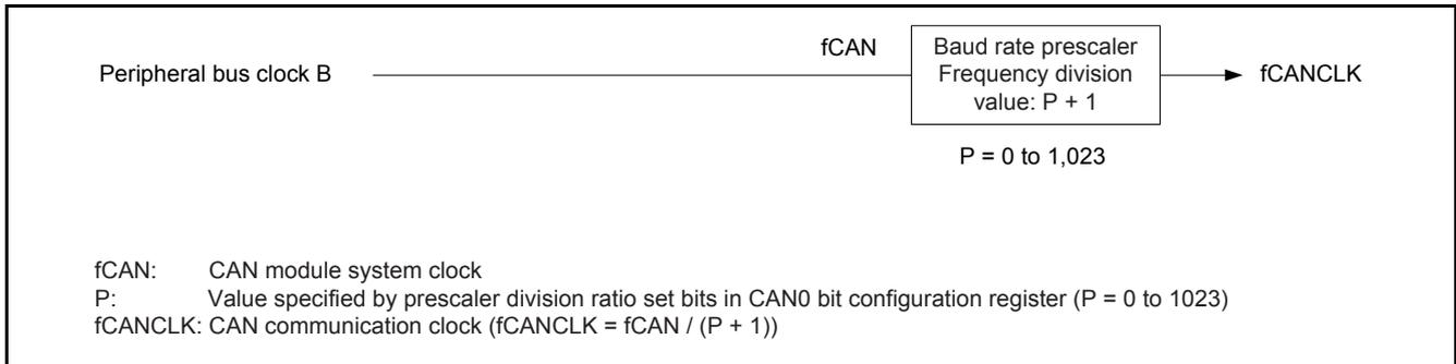
**Figure 2 Block Diagram of CAN Module System Clock Generator Circuit**
