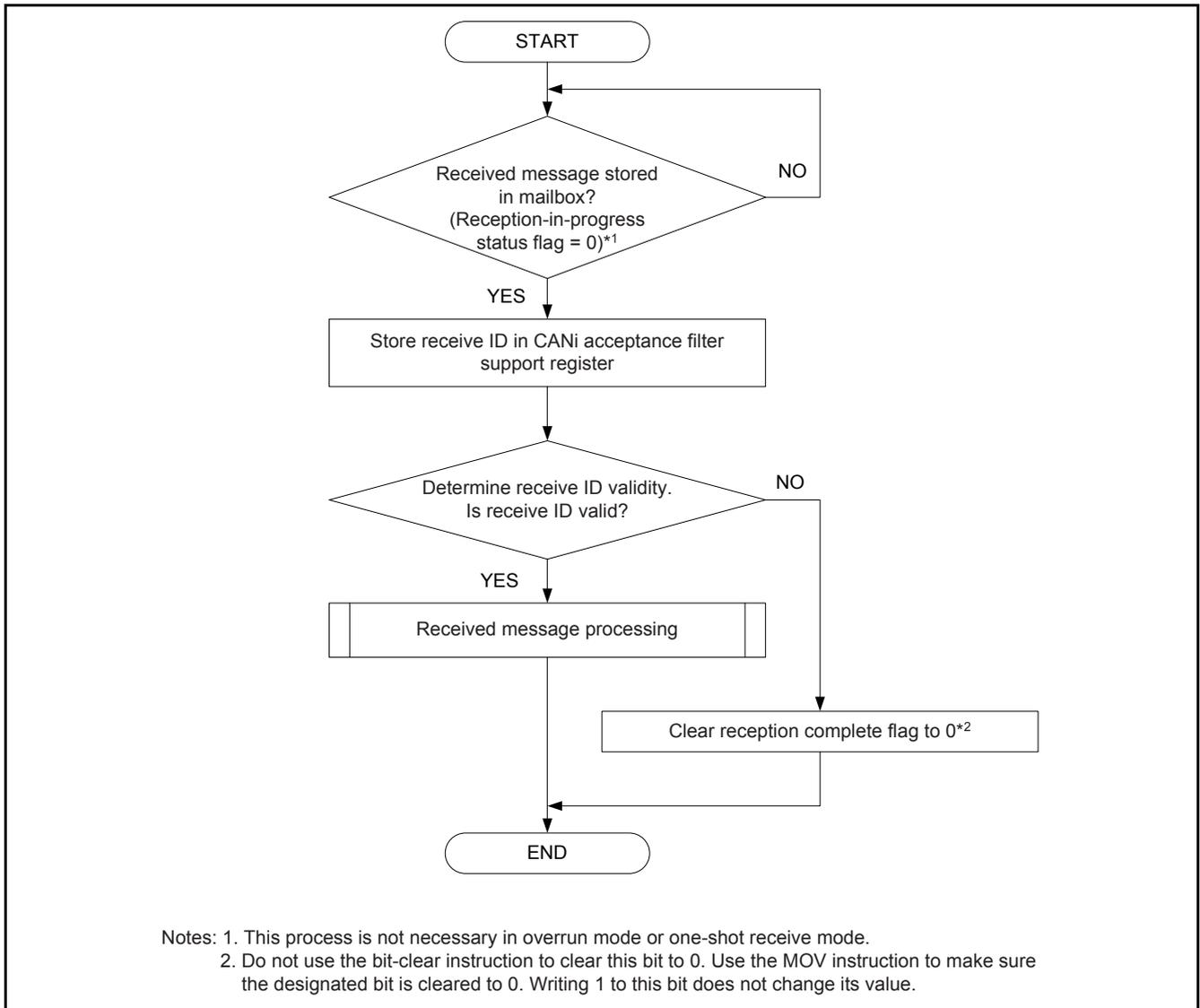
**Figure 41 Acceptance Filter Support Unit Usage Procedure**
