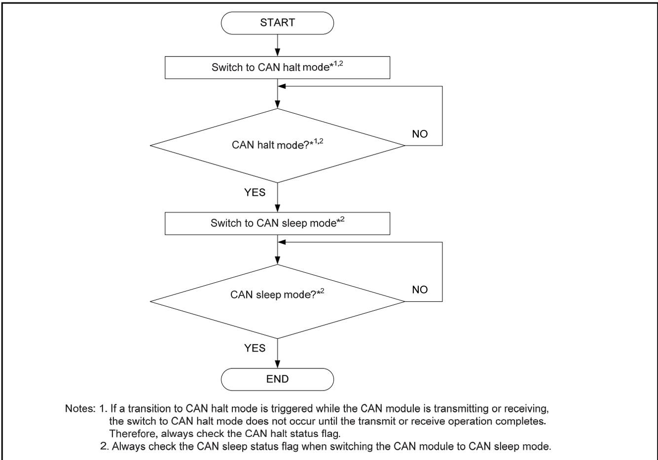
**Figure 43 Procedure for Switching CAN Module to CAN Halt Mode and then CAN Sleep Mode**
