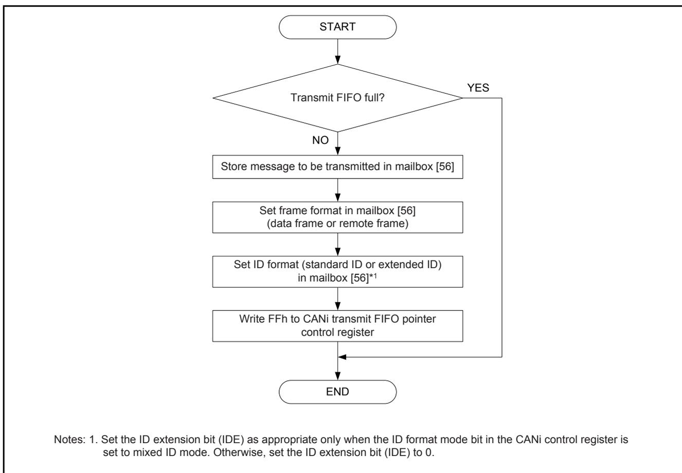
**Figure 23 Transmission Processing Procedure in FIFO Mailbox Mode**
