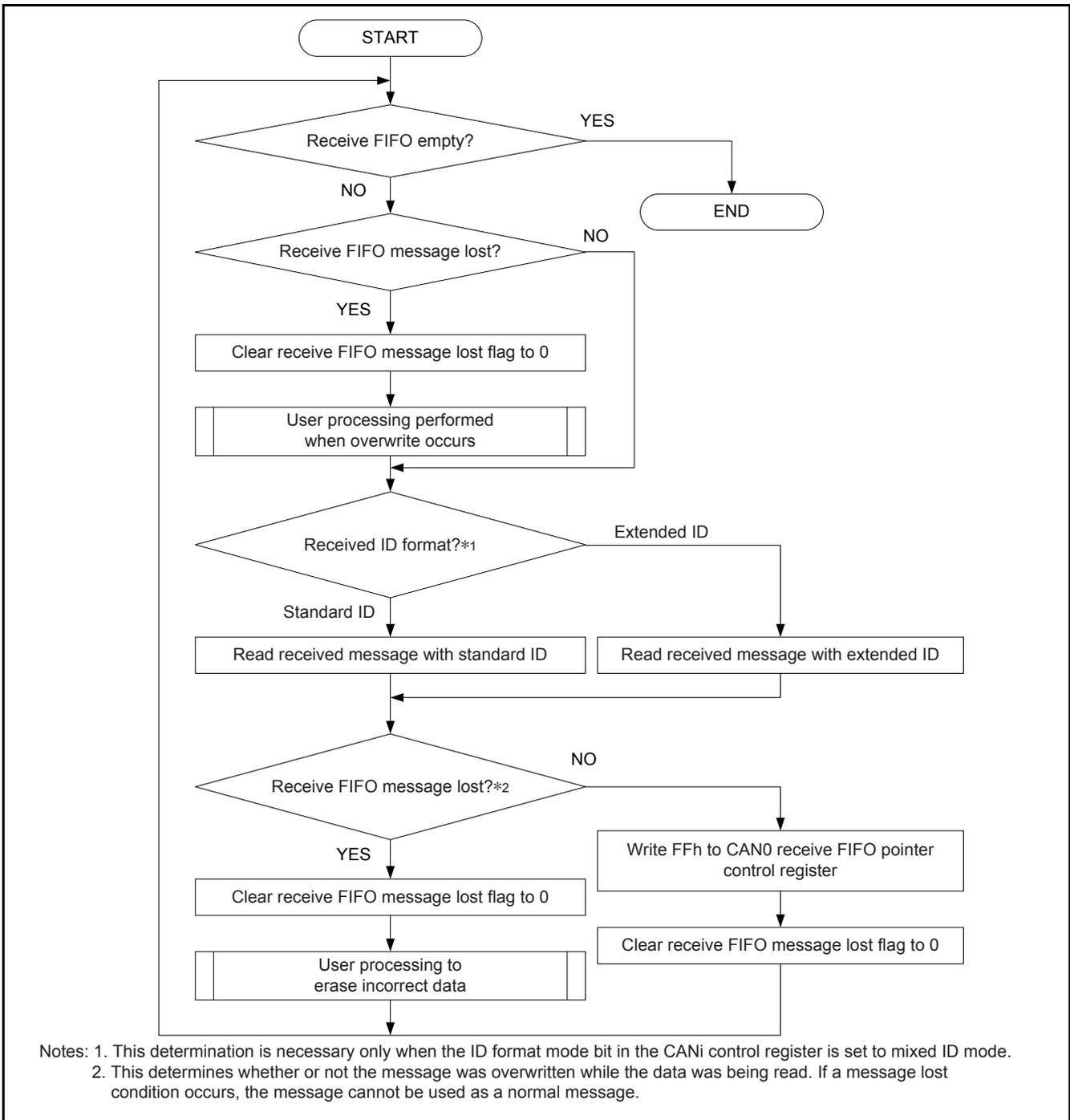
Figure 24 Reception Processing Procedure (Overwrite Mode) in FIFO Mailbox Mode
