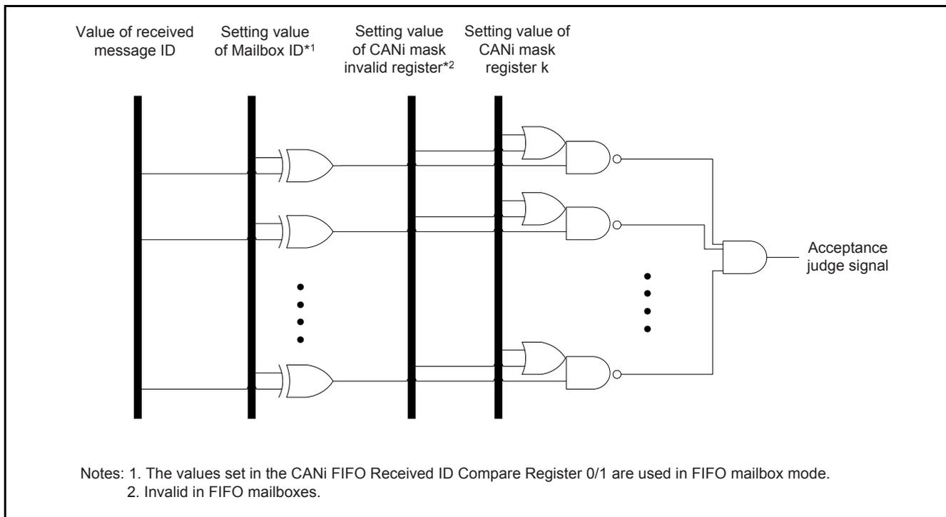
**Figure 36 ID and Mask Register Configuration**
