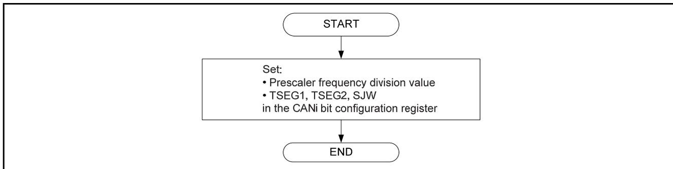
**Figure 3 CAN Bit Timing and Transfer Speed Setting Procedure**
