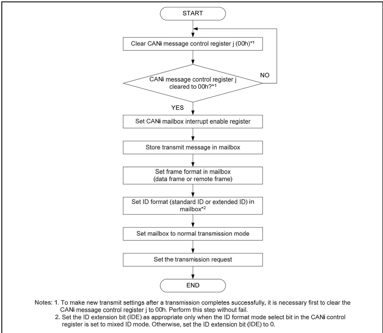
**Figure 7 Normal Transmission Request Procedure**
