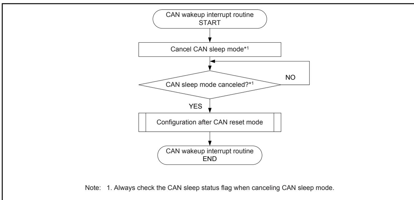
**Figure 44 CAN Wakeup Procedure in CAN Reset Mode**
