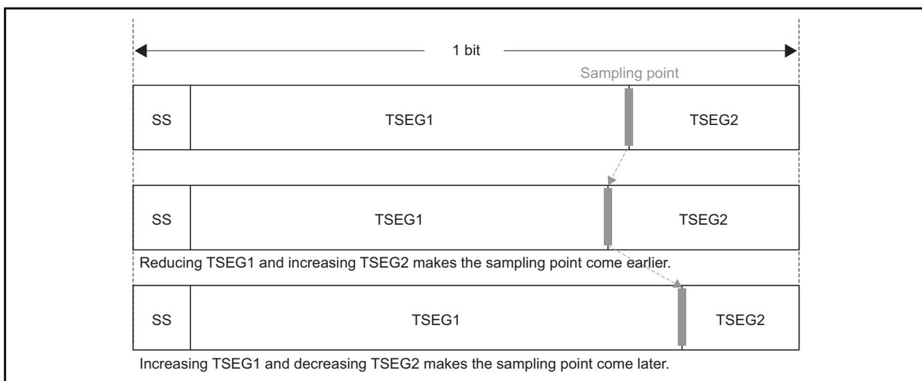
**Figure 1 Segment Structure of Bit and Sampling Point**
