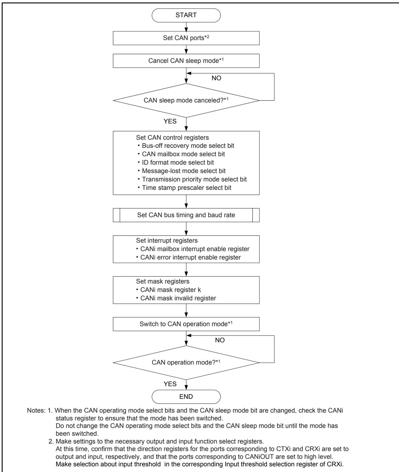
**Figure 4 CAN Configuration Procedure after a Hardware Reset**
