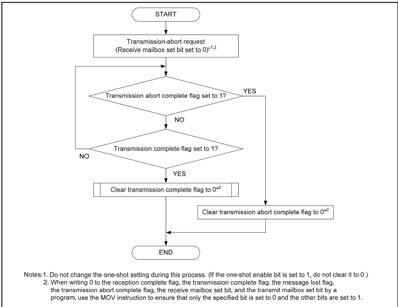
Figure 12 Transmission-Abort Procedure
