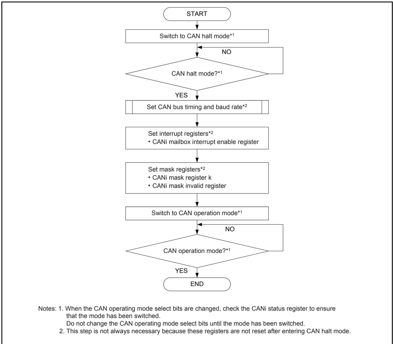
**Figure 6 CAN Configuration Procedure after Transitioning to CAN Halt Mode**
