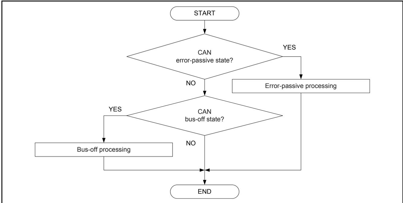
Figure 32 CAN Error State Checking Procedure (Using Polling)
