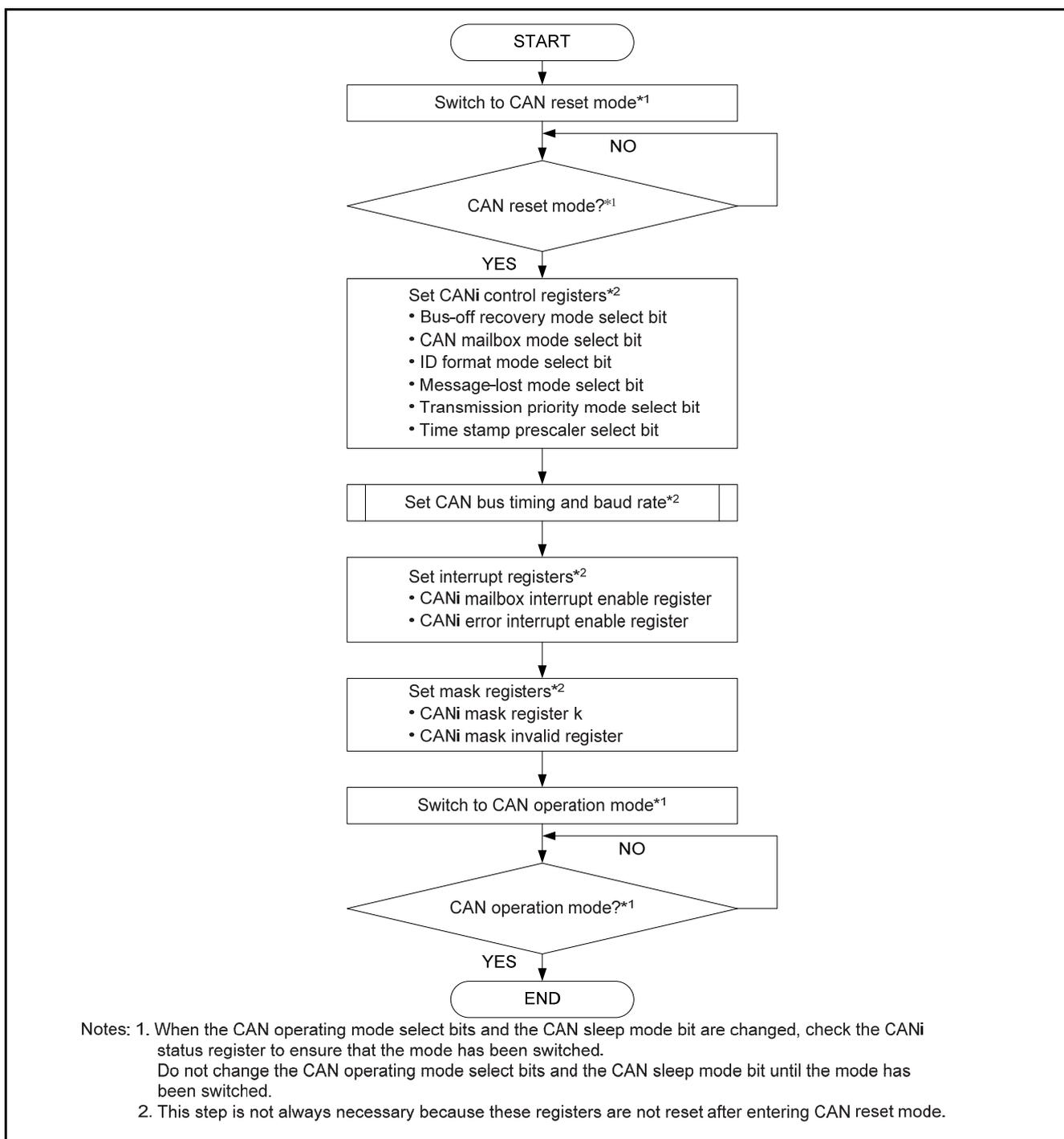
**Figure 5 CAN Configuration Procedure after Transitioning to CAN Reset Mode**
