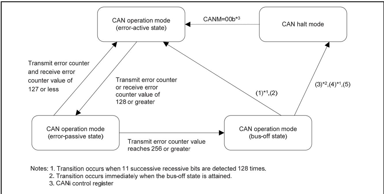
Figure 34 Transition to and from the Bus-Off State
