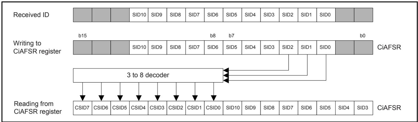
Figure 40 States when Writing to and Reading from CANi Acceptance Filter Support Register
