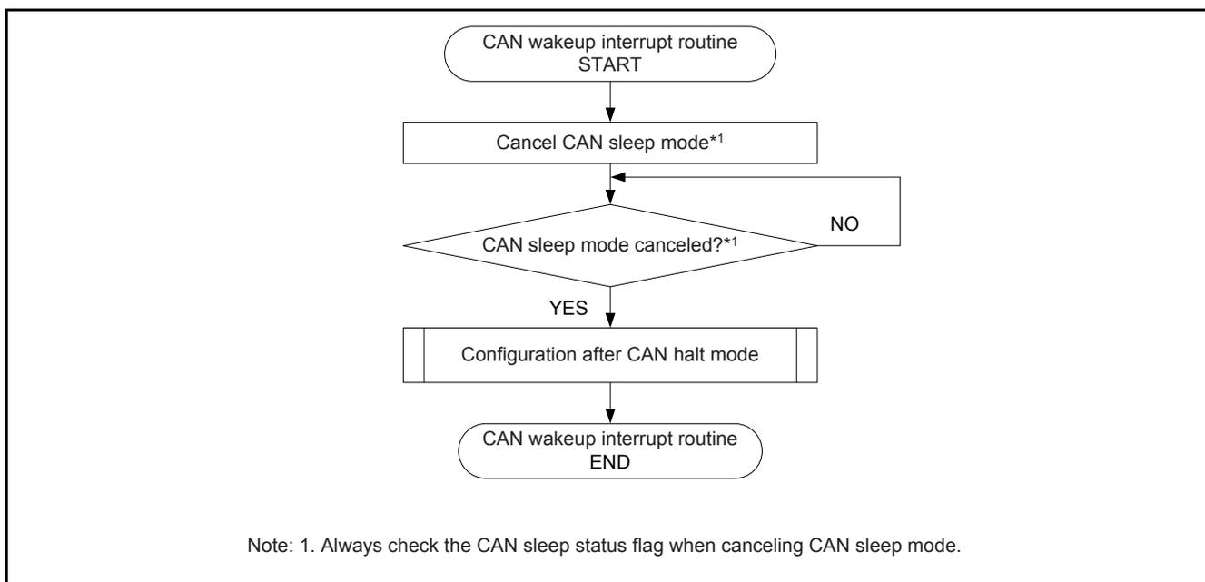
**Figure 45 CAN Wakeup Procedure in CAN Halt Mode**
