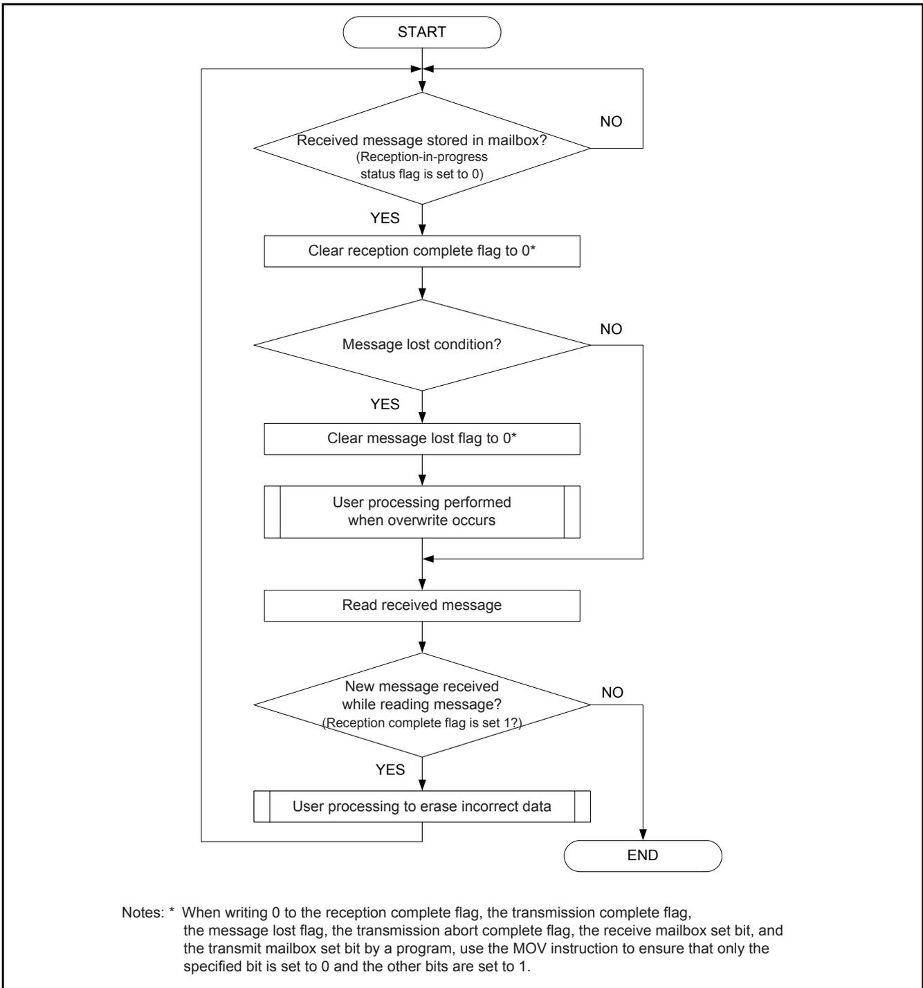
**Figure 14 Message Reception Processing with Mailbox Set to Normal Reception Mode (Overwrite Mode)**
