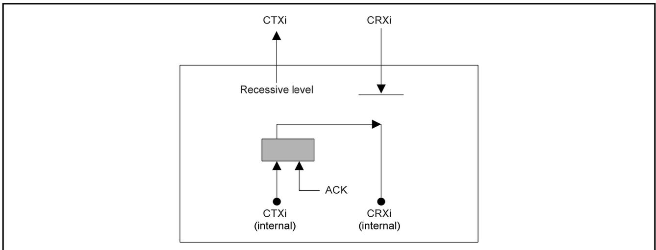
Figure 49 Self-Test Mode 1 Operation Illustration
