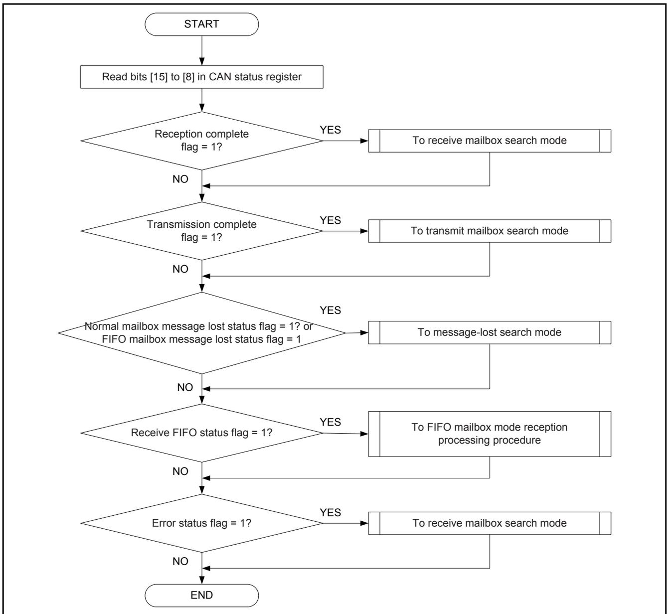
Figure 26 CAN Status Register Checking Example (Polling Operation)
