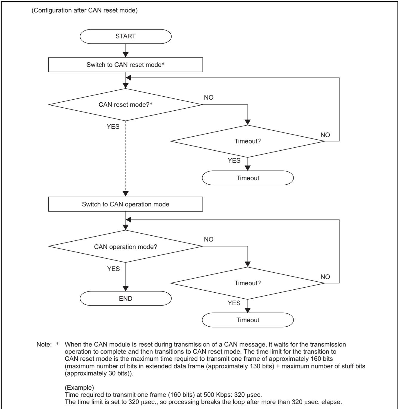
Figure 50 Processing Example with Loop Time Limit
