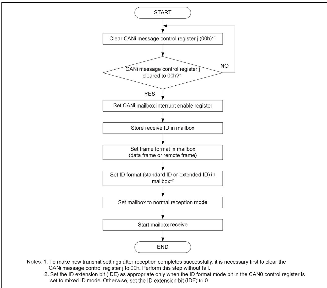
**Figure 13 Normal Reception Request Procedure**
