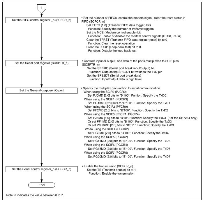
Figure 3 Flow Chart for Configuring the Transmission in Asynchronous Mode (2/2)
