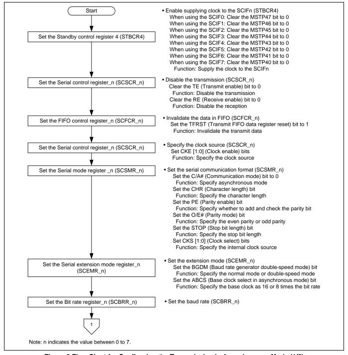
Figure 2 Flow Chart for Configuring the Transmission in Asynchronous Mode (1/2)
