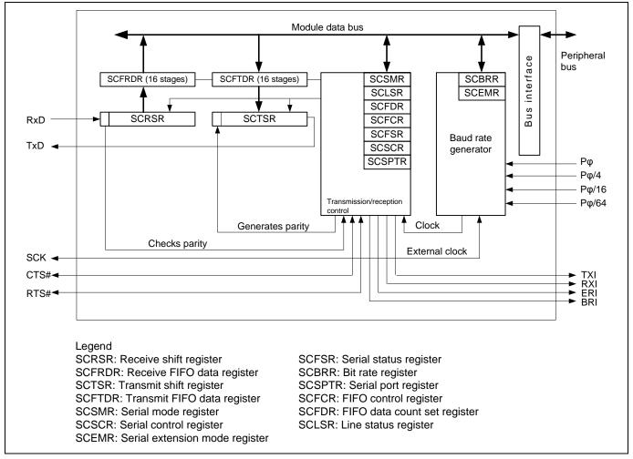
Figure 1 SCIF Block Diagram
