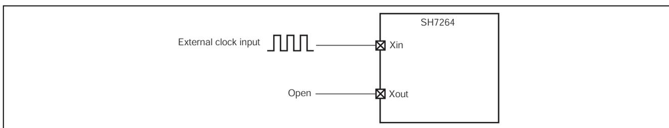
**Figure 6 Connecting an External Clock**
