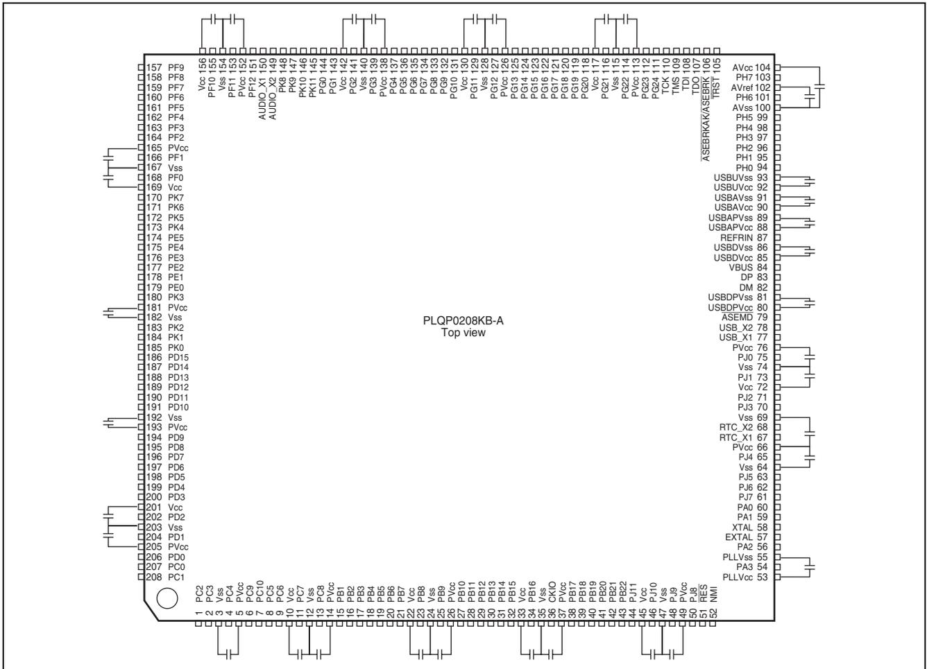
Figure 3 Installing an External Capacitor with the SH7264
