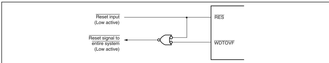
Figure 5: System Reset using WDTOVF#
