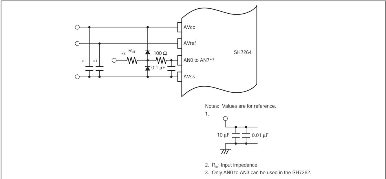
Figure 15 Analog Input Pin Protection Circuit Example
