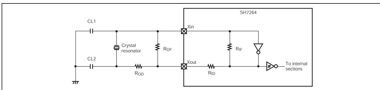
Figure 7 Connecting a Crystal Resonator
