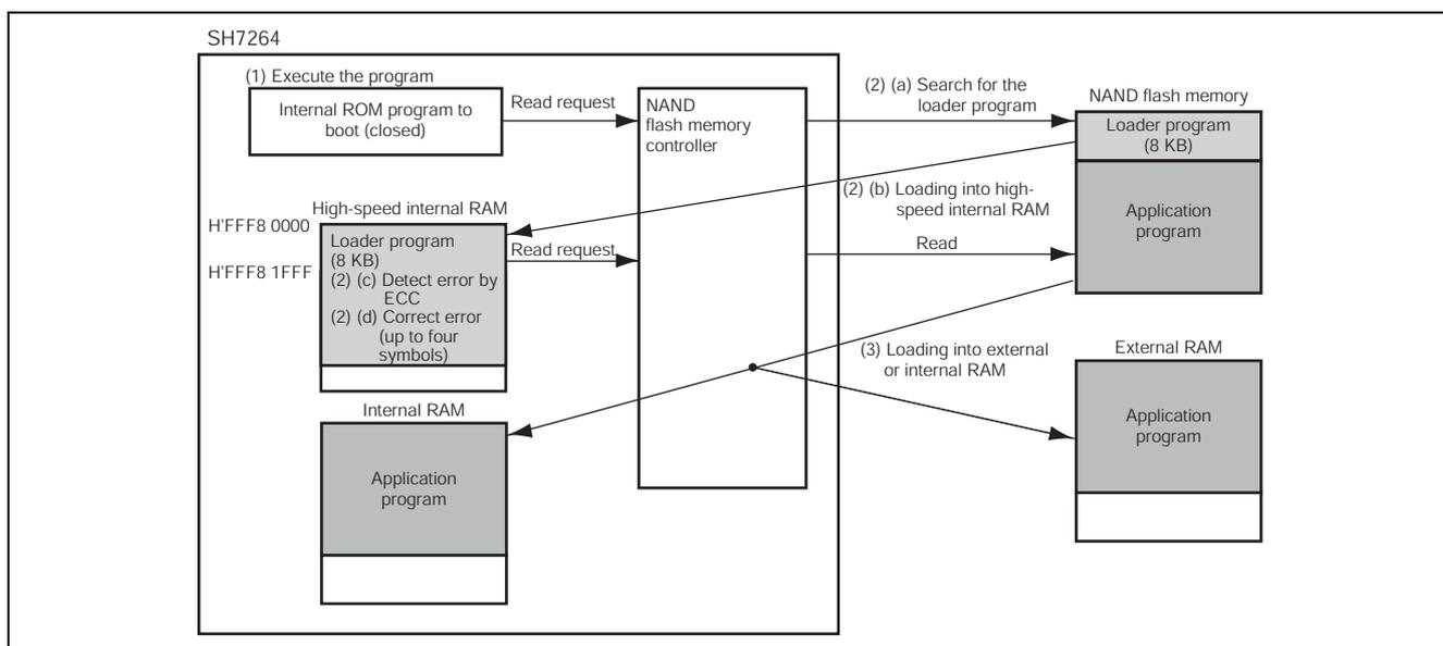
Figure 9 Boot Mode 2 Schematic View
