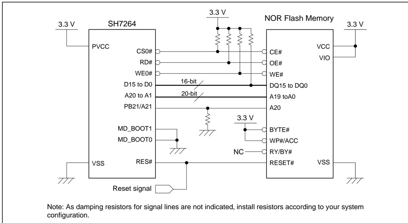
Figure 10 Typical NOR Flash Memory Circuit
