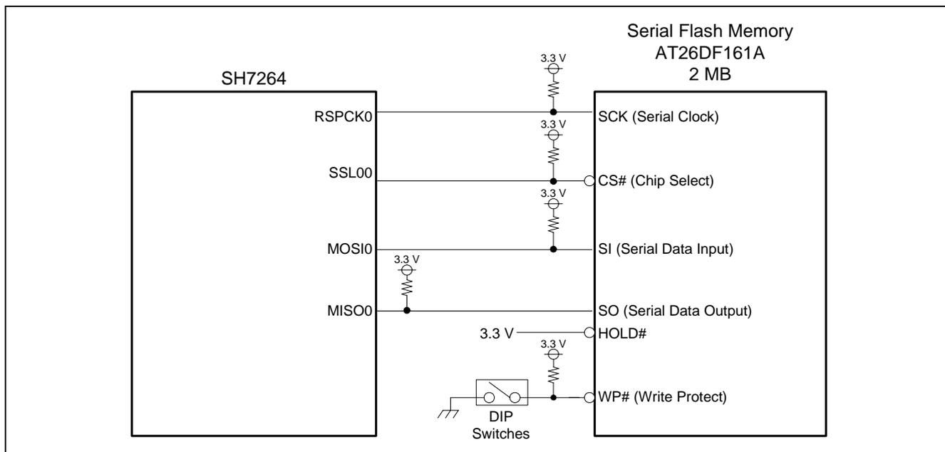
**Figure 11 Typical Serial Flash Memory Circuit**
