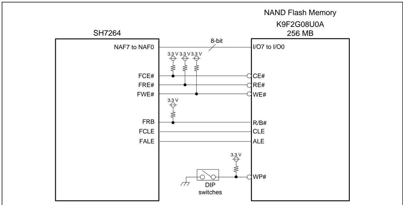
**Figure 12 Typical NAND Flash Memory Circuit**
