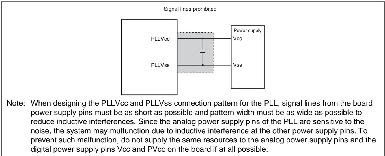
**Figure 1 Note on Using PLL Oscillation Circuit**
