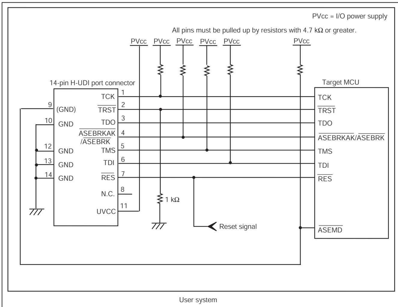
Figure 14 Recommended Circuit between the 14-pin H-UDI Port Connector and MCU (with E10A-USB)
