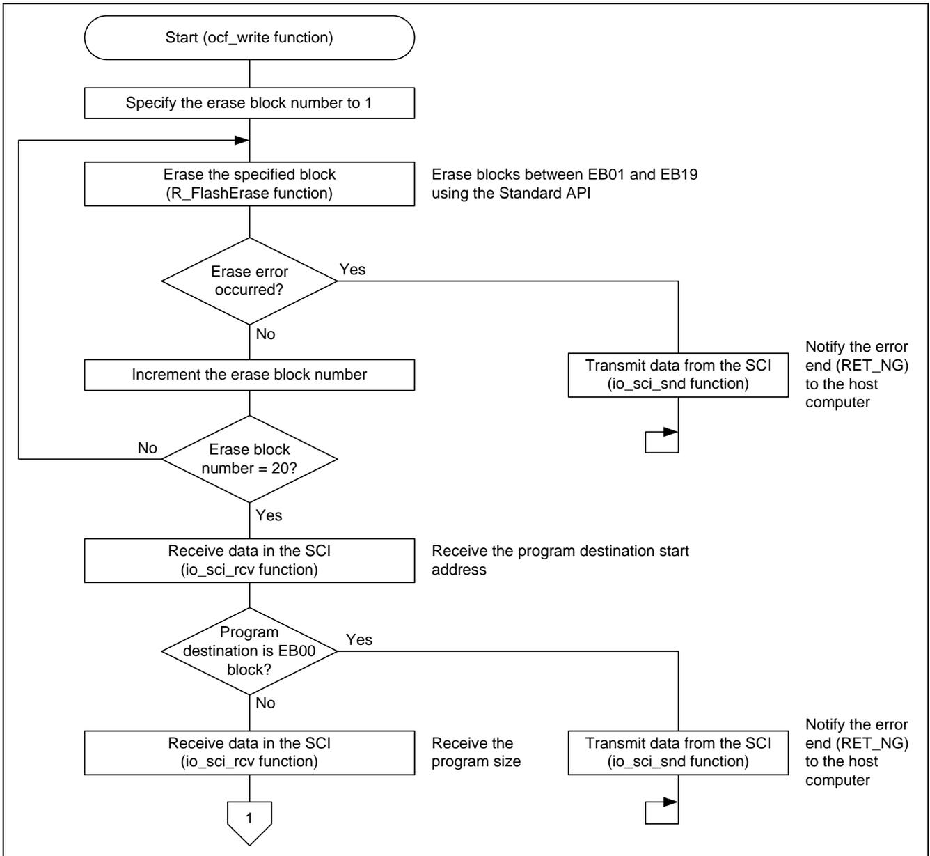
Figure 15 Programming/Erasing the Flash Memory (1/2)
