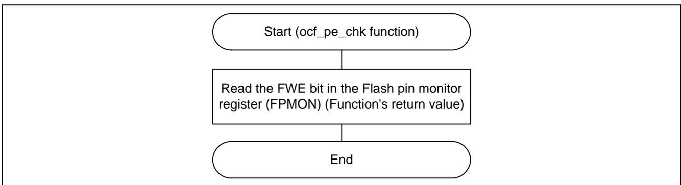
Figure 18 Checking the Flash Memory is Program-/Erase-enabled
