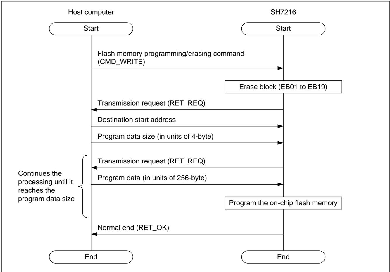
Figure 12 Communication Command Sequence When Programming/Erasing the Flash Memory
