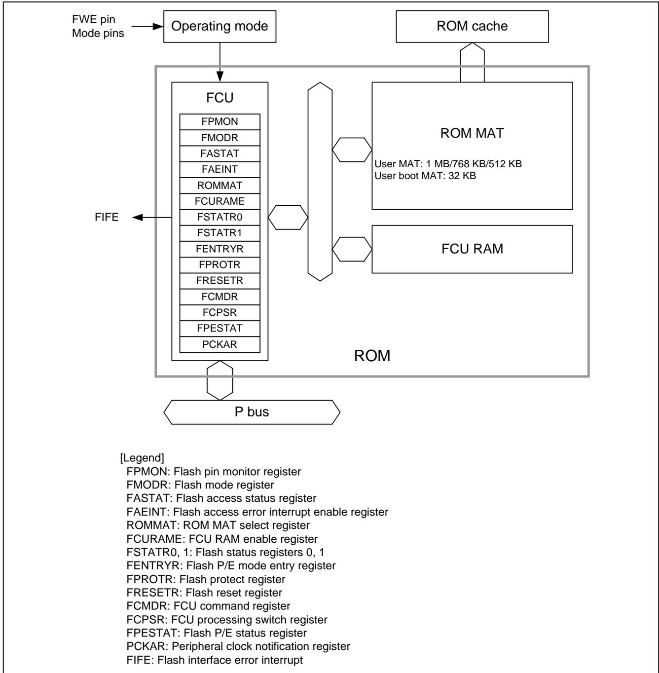
**Figure 3 Flash Memory Block Diagram**
