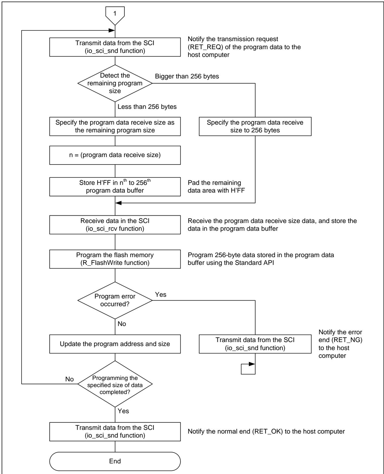
Figure 16 Programming/Erasing the Flash Memory (2/2)
