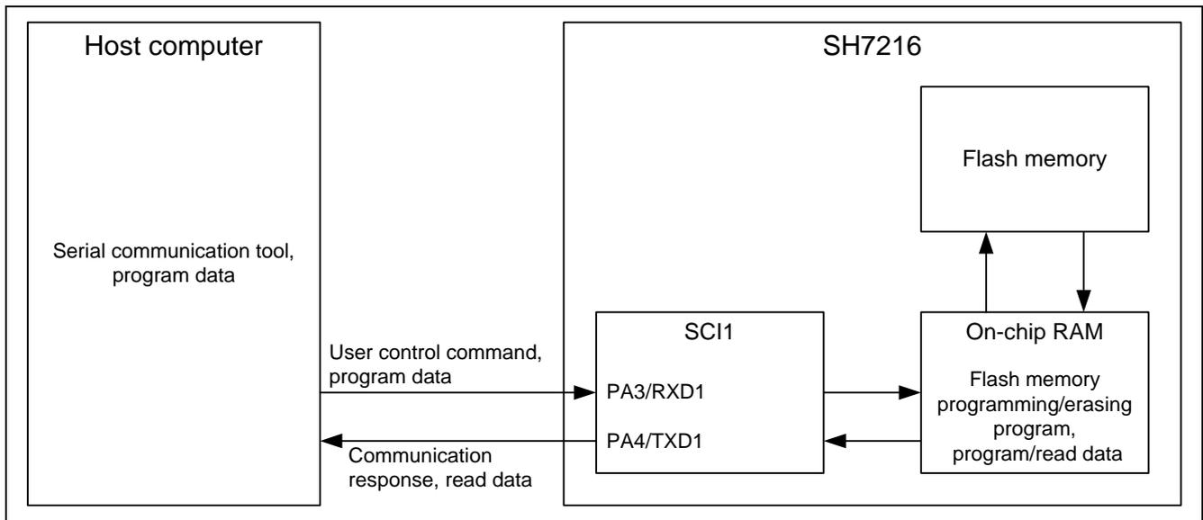
Figure 1 System Configuration
