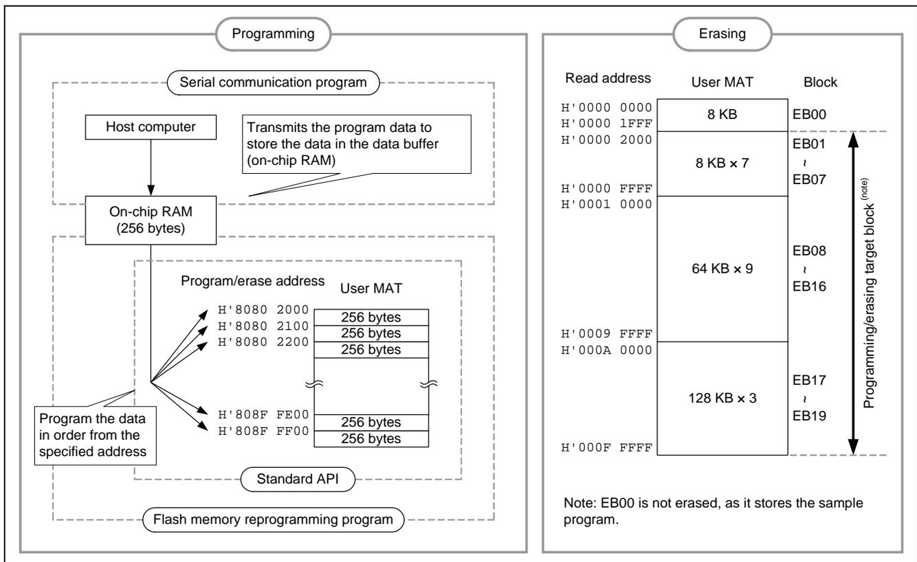
Figure 10 Programming and Erasing the Flash Memory
