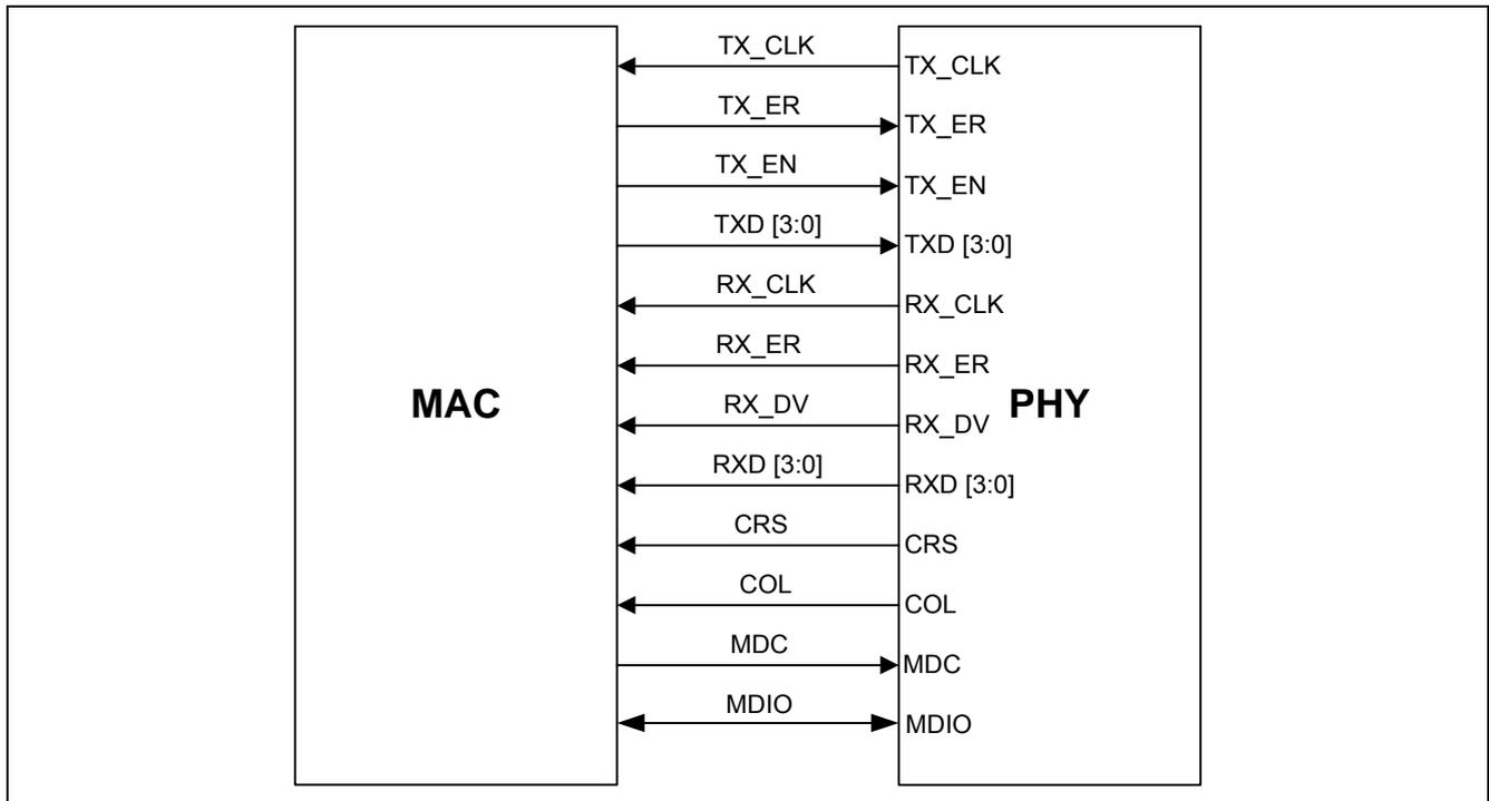
Figure 1 MII Signal Connection
