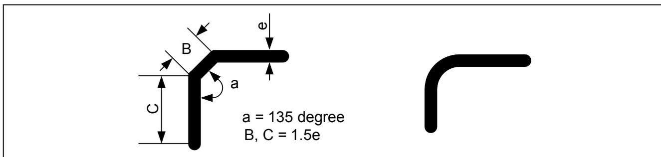
Figure 3 Wiring Corner Angle
