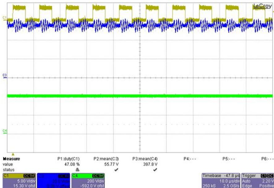
Figure 7 Output power is 1400 W at 3.5 A
