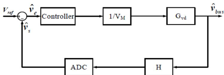
Figure 3 PI algorithm for boost
