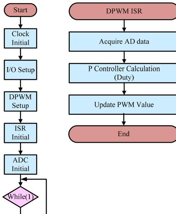
Figure 5 Flow chart for Step-Up Boost
