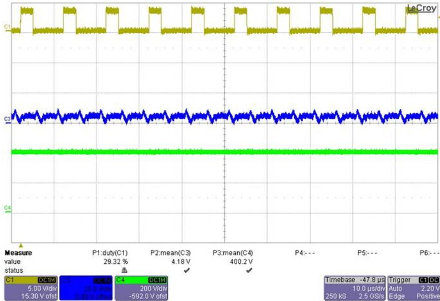
Figure 6 Output power is 108 W at 0.25 A
