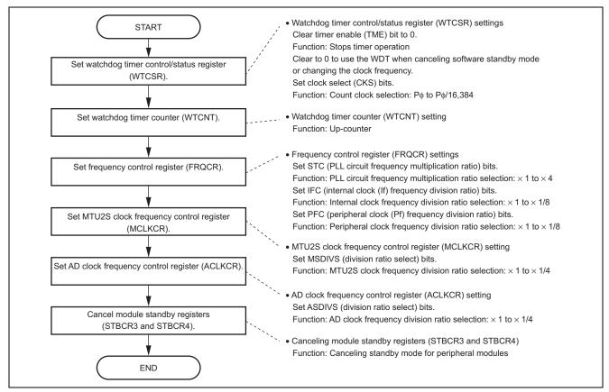
Figure 3 Example Settings Sequence for Changing Operating Frequency
