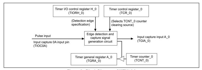
Figure 2 Block Diagram of MTU/ch0
