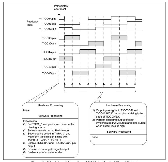
Figure 3 Principles of Operation of DC Motor Control Signal Output
