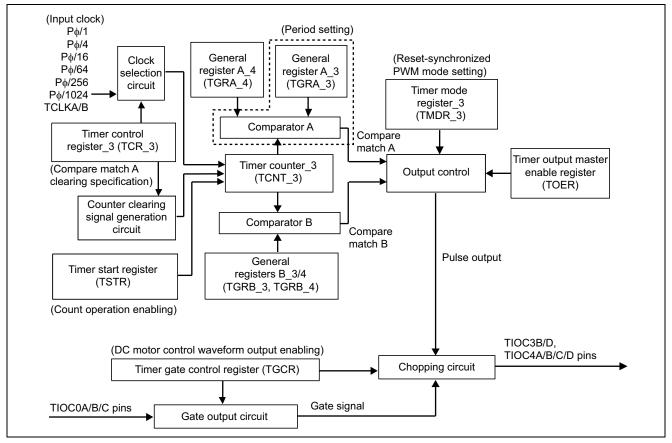
Figure 2 Block Diagram of MTU/ch3, ch4
