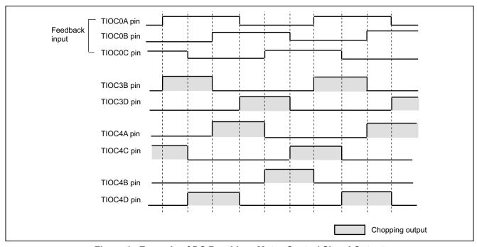
Figure 1 Example of DC Brushless Motor Control Signal Output
