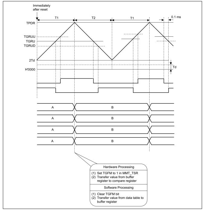
Figure 5 Principles of Operation of Complementary PWM U-Phase Waveform
