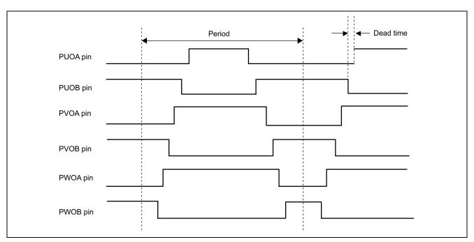
Figure 1 Complementary PWM 3-Phase Output Waveforms
