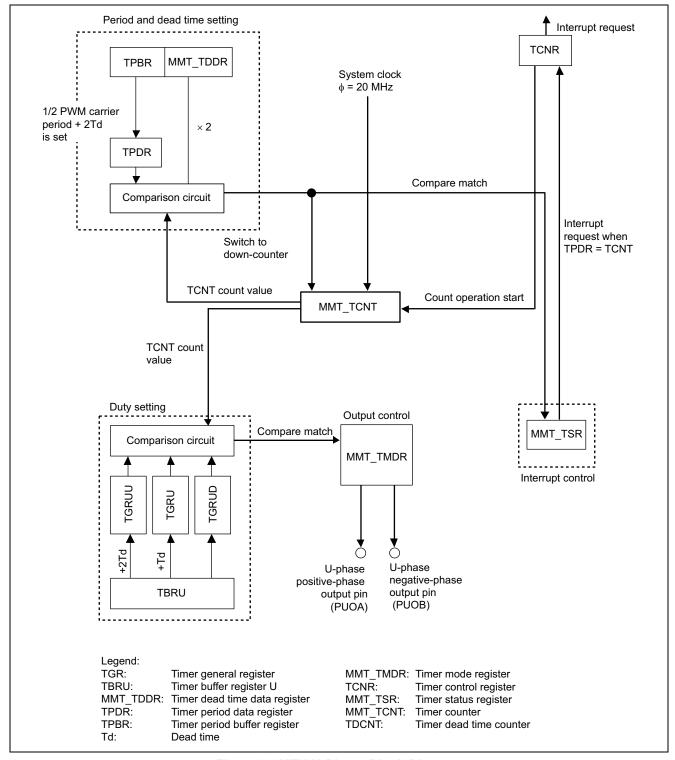
Figure 2 MTU U-Phase Block Diagram
