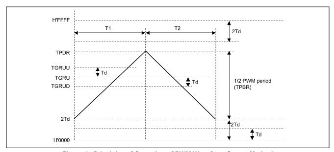
Figure 4 Principles of Operation of PWM Waveform Output Method
