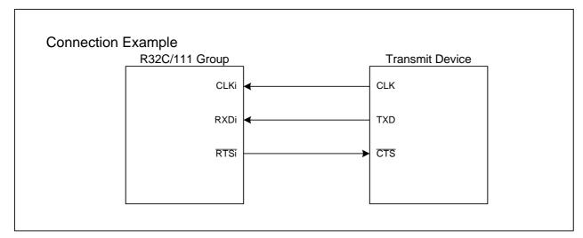
Figure 3.1 Receive Connection Example
