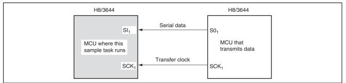
Figure 1.1 Serial Data Reception in Synchronous Mode
