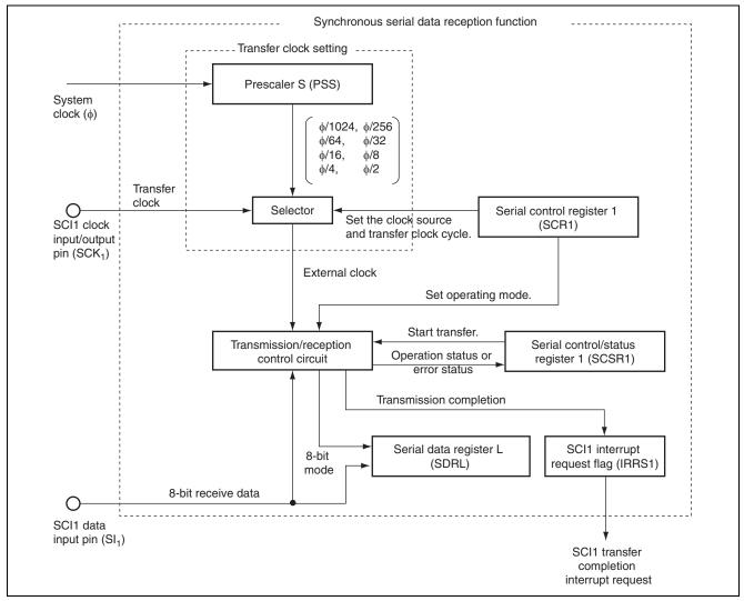
Figure 2.1 Block Diagram of Synchronous Serial Data Reception Function
