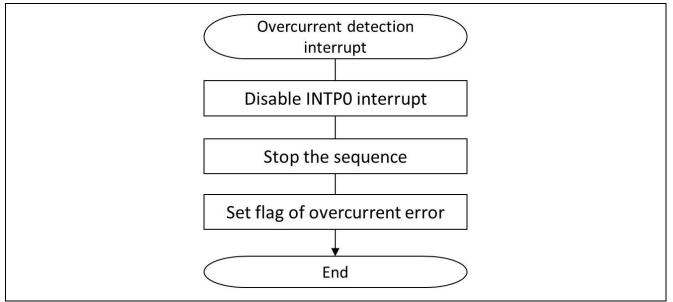
Figure 3-12 Over Current Detection Interrupt Handling
