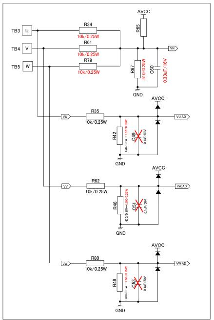
Figure 1-2 Modification for the circuit to sensing voltage of each phase
