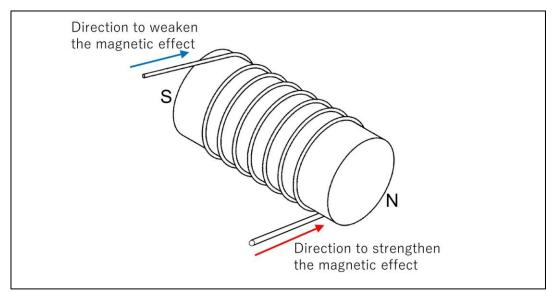
Figure 3-5 Example of a magnet with winding a coil
