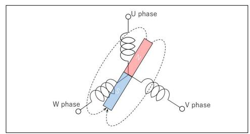
Figure 3-1 Relation between the rotor's angle and each phase
