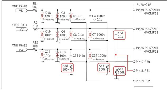
Figure 1-3 Modification of CPU card (T5103)
