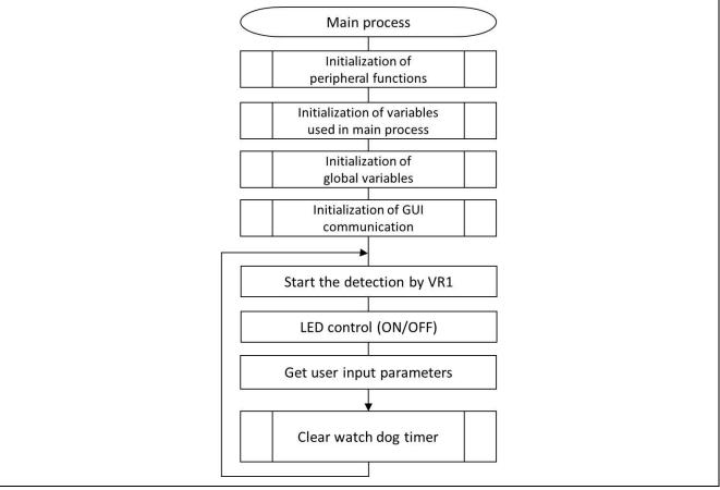
**Figure 3-9 Main Process Flowchart**
