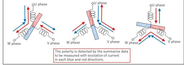
Figure 3-7 Pattern of current to arise the magnetic saturation (sample)
