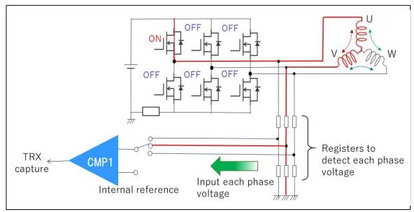
Figure 3-2 Pattern diagram to estimate the rotor's angle
