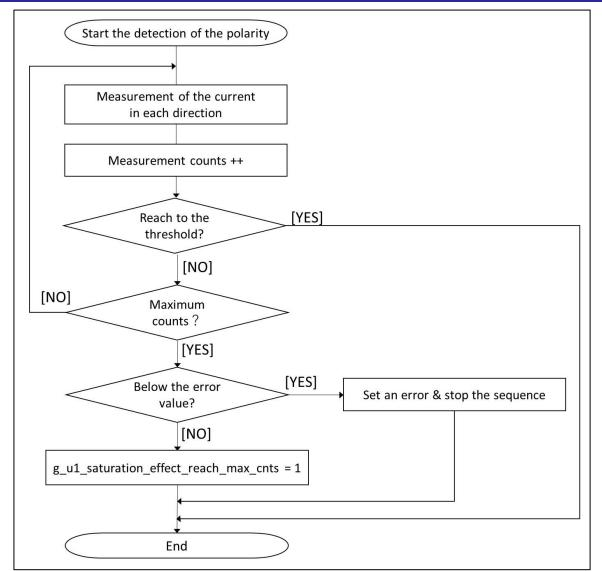
Figure 3-8 Flowchart of the detection of the polarity
