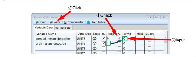
Figure 4-2 Procedure – Start the detection
