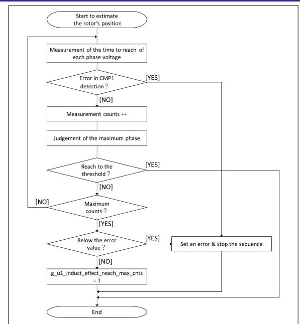
Figure 3-4 Flowchart of the estimation of the rotor's angle
