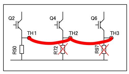
Figure 1-1 Change 3-shunt to 1-shunt
