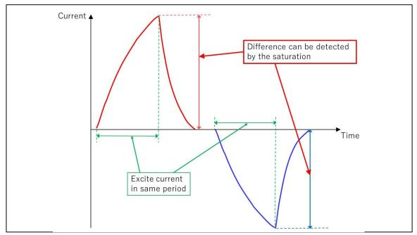
Figure 3-6 Difference of current between the excited direction
