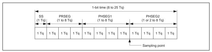
Figure 4 Configuration of One-Bit Time
