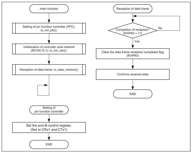
Figure 6 Example of Flow of Processing by the Sample Program
