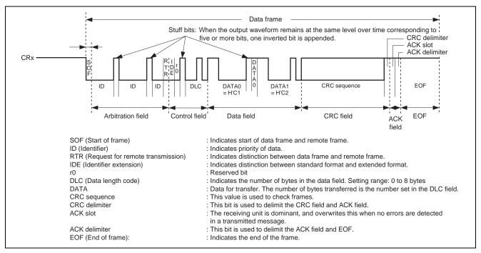
Figure 5 Waveform for Data Frame Reception by the RCAN-TL1
