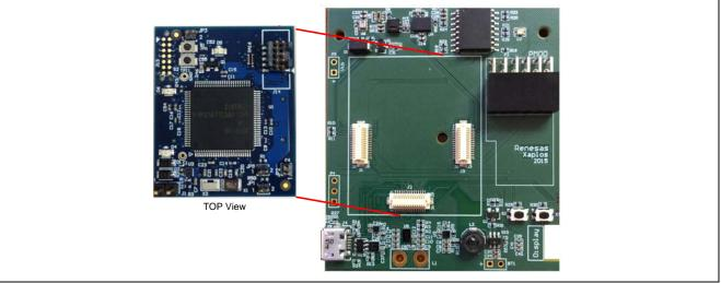
Figure 2 Example of S3 Series Board interface pin configuration with an Activity Module
