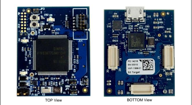
Figure 1 Synergy S3 Series Module
