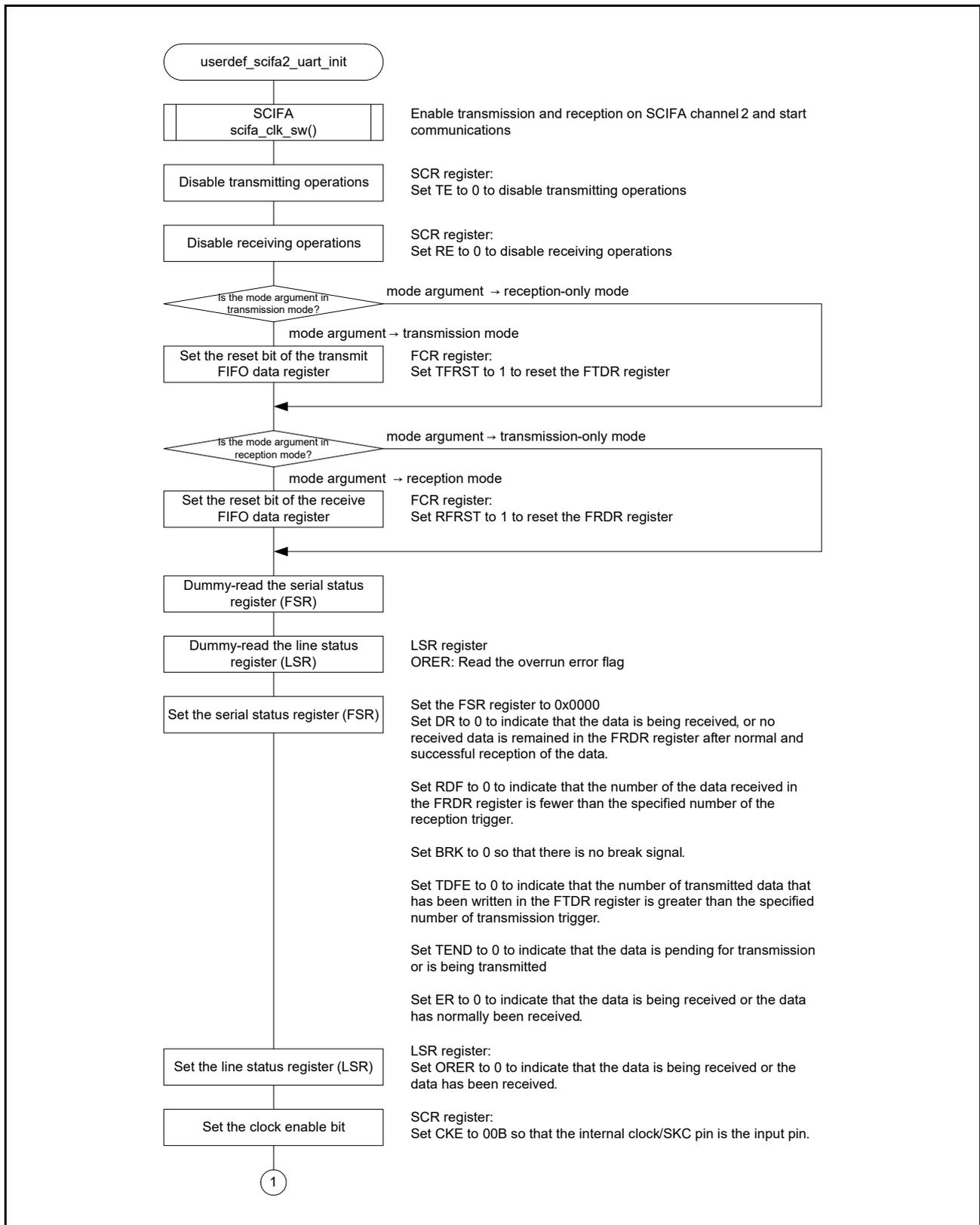
Figure 6.10 Initialization of SCIFA Channel 2 in UART Mode (User Defined) (1)
