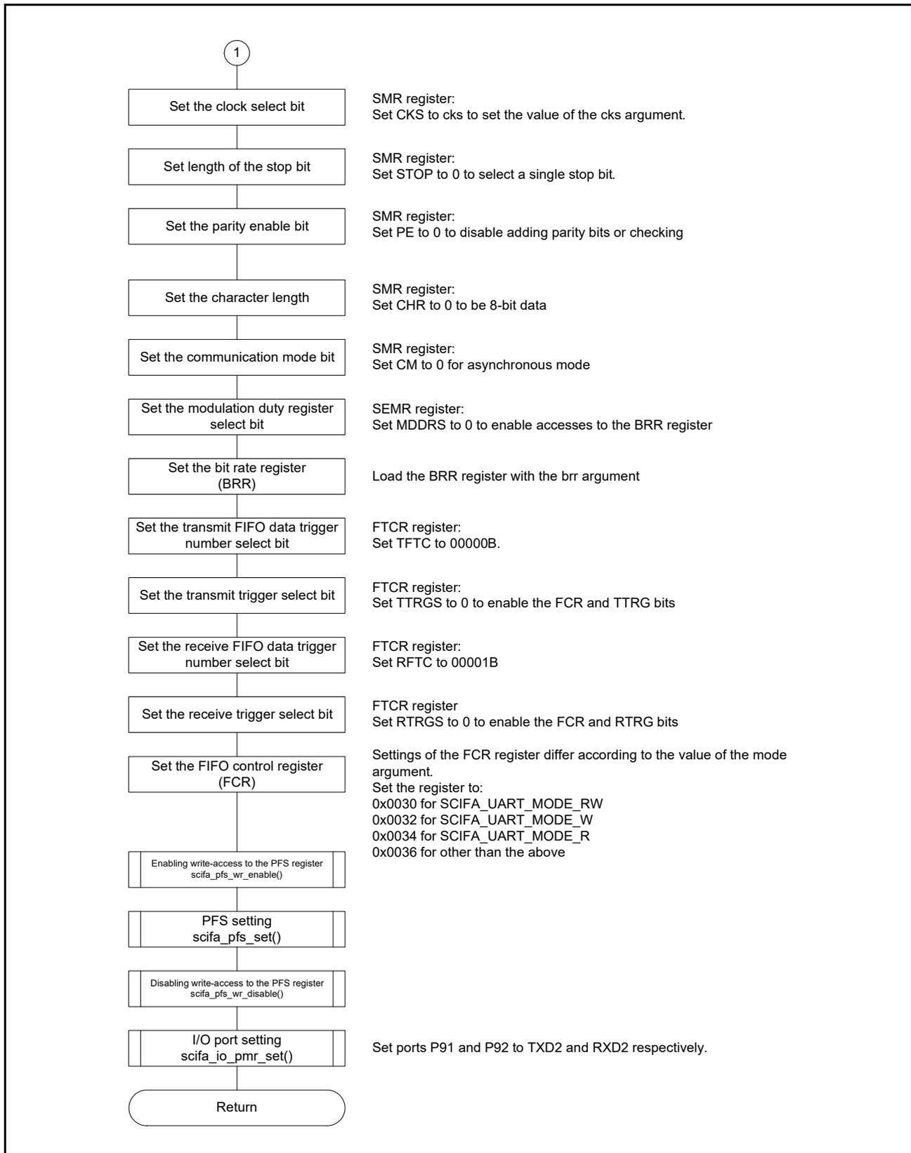
Figure 6.11 Initialization of SCIFA Channel 2 in UART Mode (User Defined) (2)
