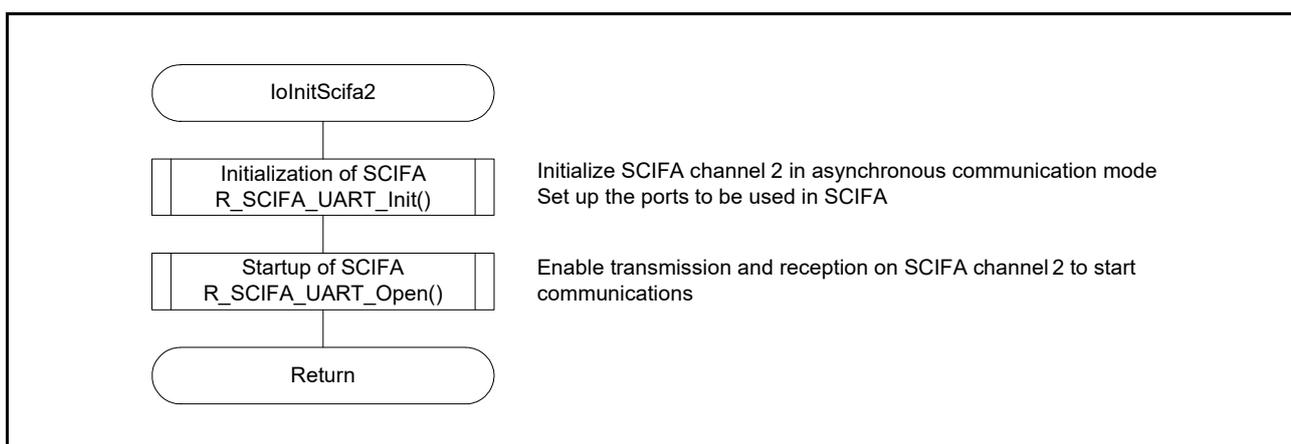
Figure 6.5 Initialization of SCIFA Channel 2
