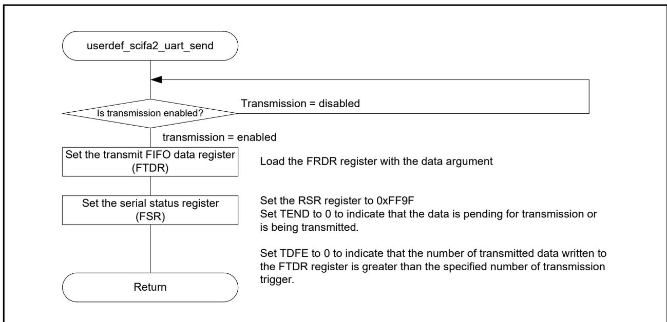
Figure 6.13 Transmission of SCIFA Channel 2 (User Defined)
