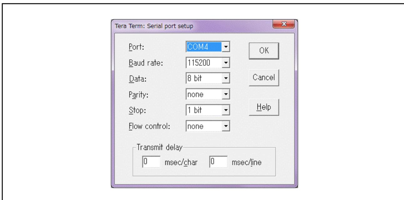
Figure 6.1 Settings of Serial Port
