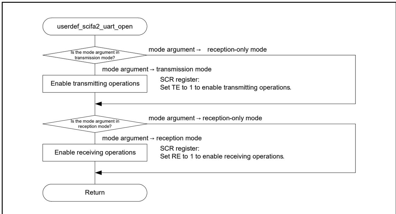
Figure 6.12 Startup of SCIFA Channel 2 in UART Mode (User Defined)
