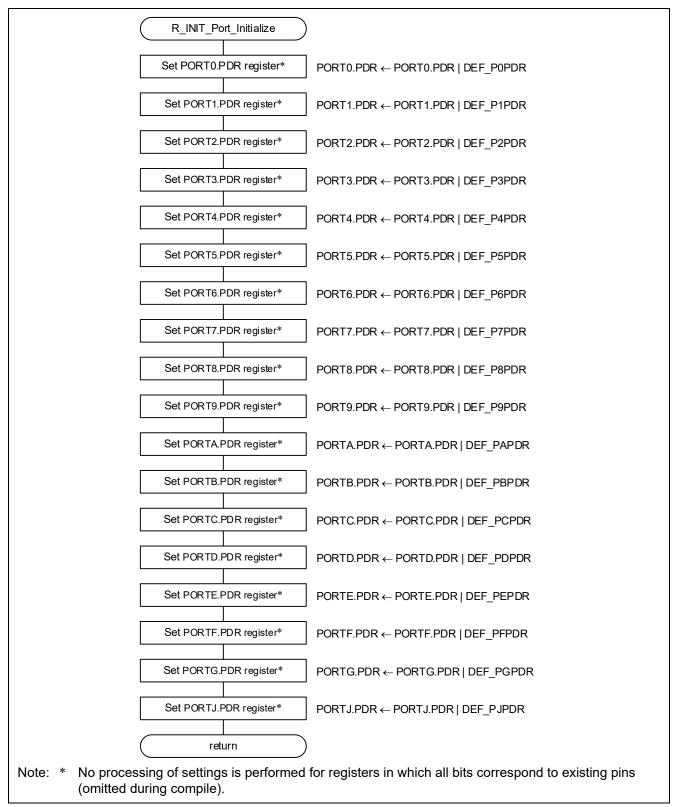
Figure 3.3 Initial Nonexistent Port Settings
