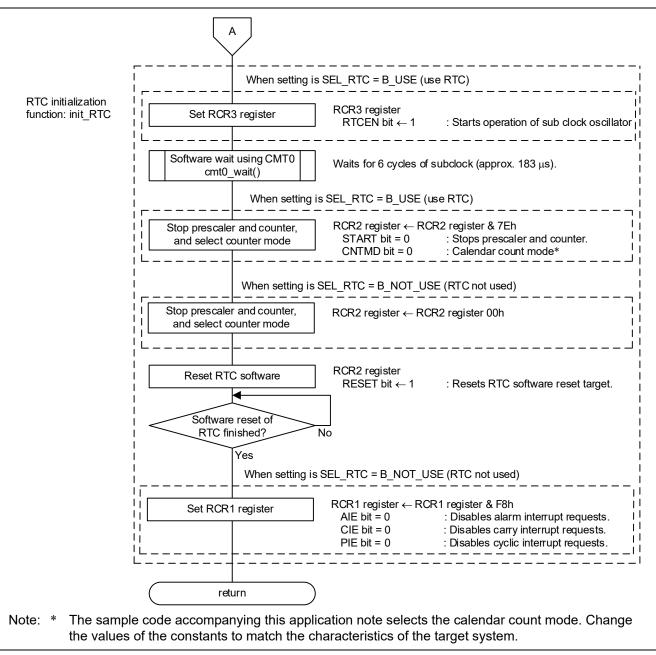
Figure 3.10 Sub-clock Oscillation Enable (2/2)
