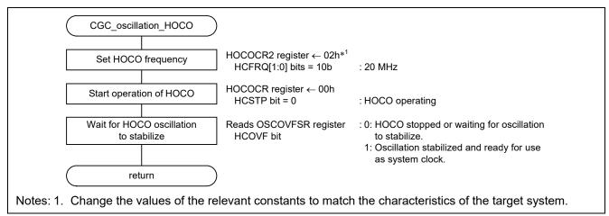
Figure 3.8 HOCO Clock Oscillation Enable
