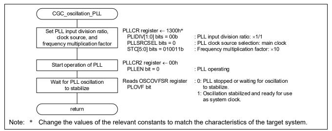
Figure 3.7 PLL Clock Oscillation Enable
