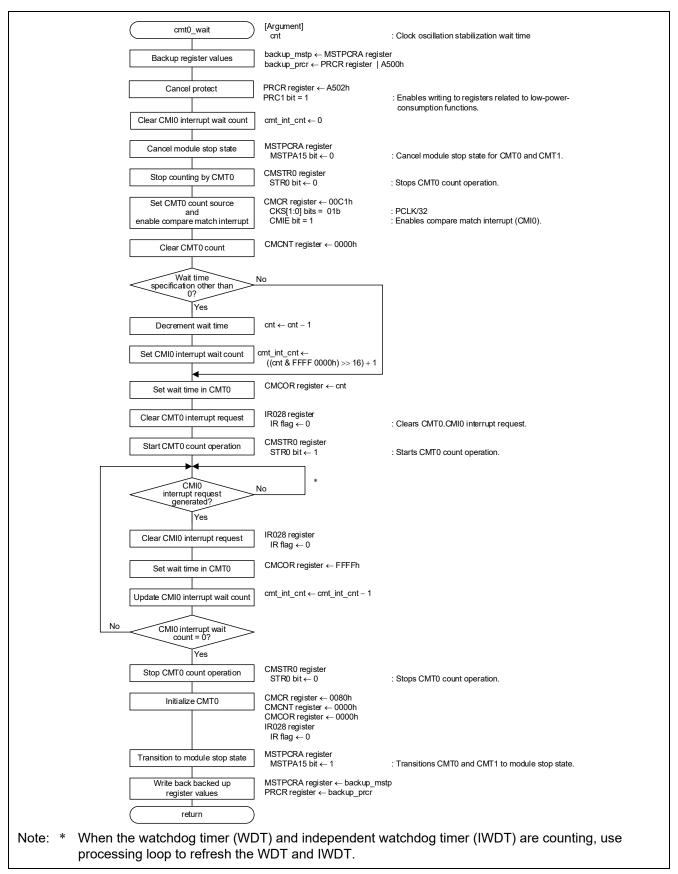
Figure 3.12 Software Wait Cycles Using CMT0
