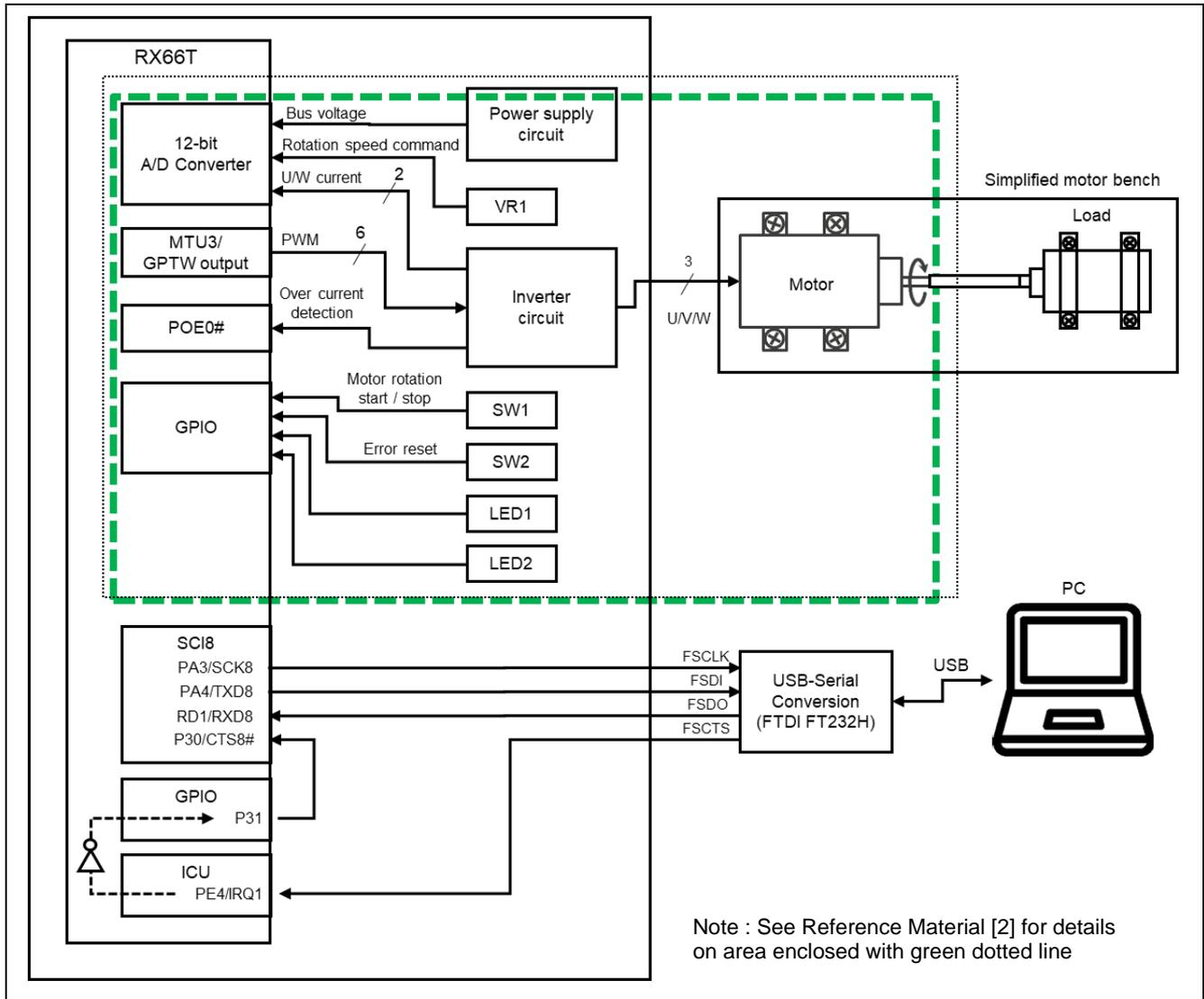
Figure 3-1. Hardware Block Diagram
