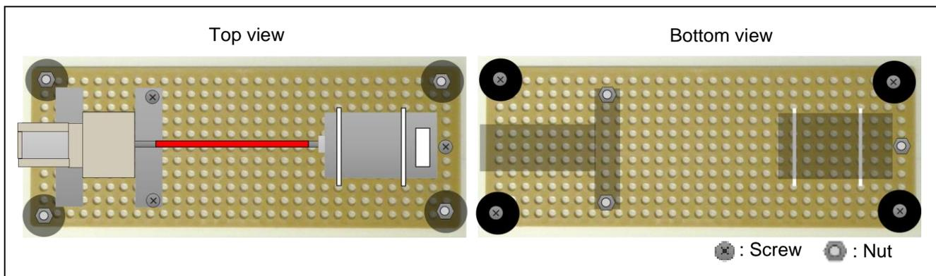
Figure 2. Simple motor bench - Parts location
