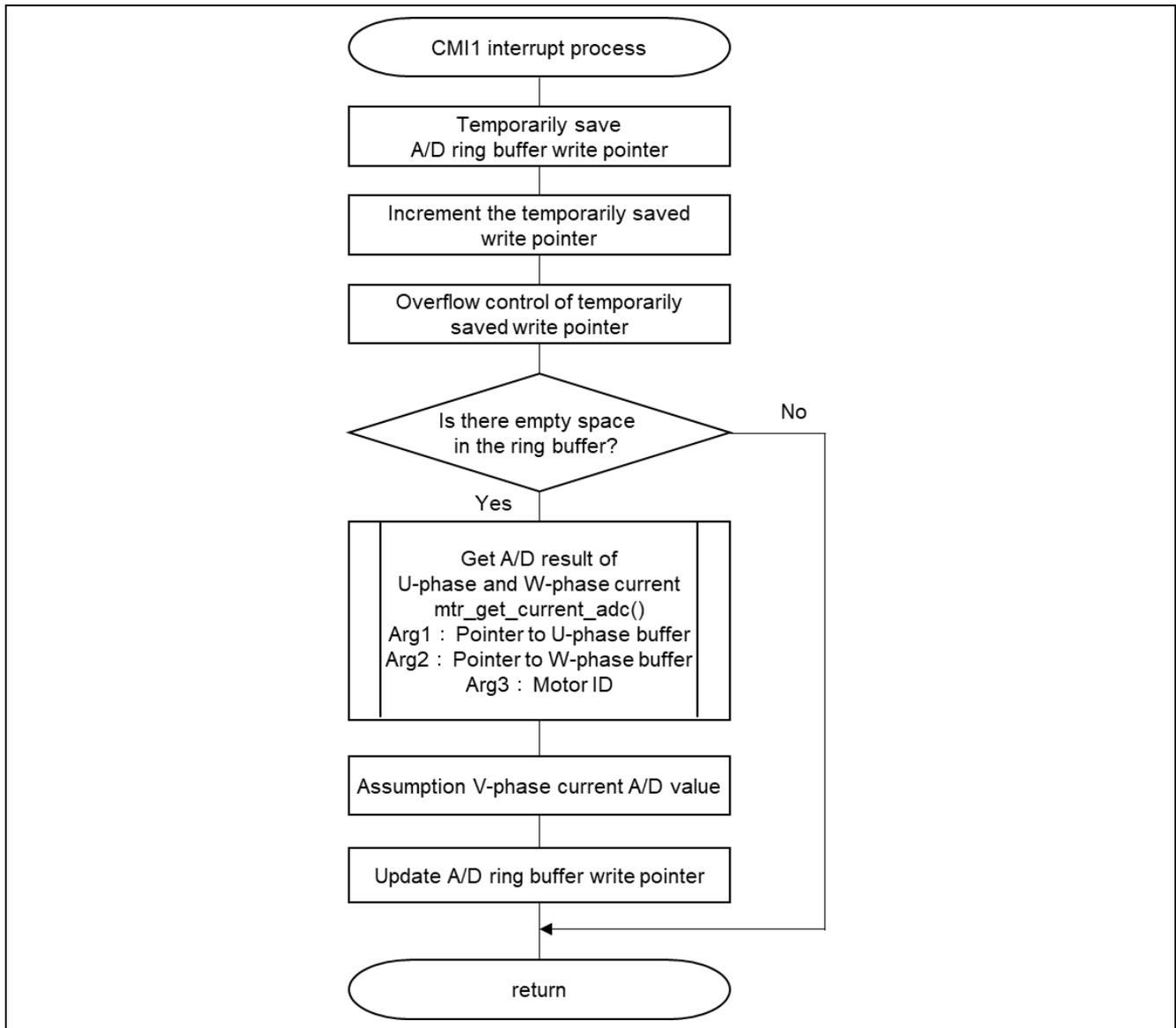
Figure 4-5. Flowchart for getting A/D conversion result of motor current value
