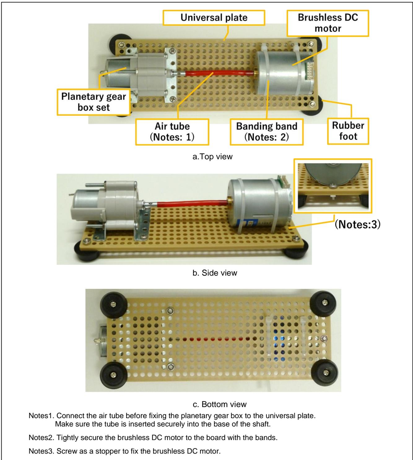
**Figure 1. Simple motor bench - Appearance**
