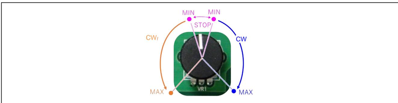
Figure 8. Control of motor rotation speed
