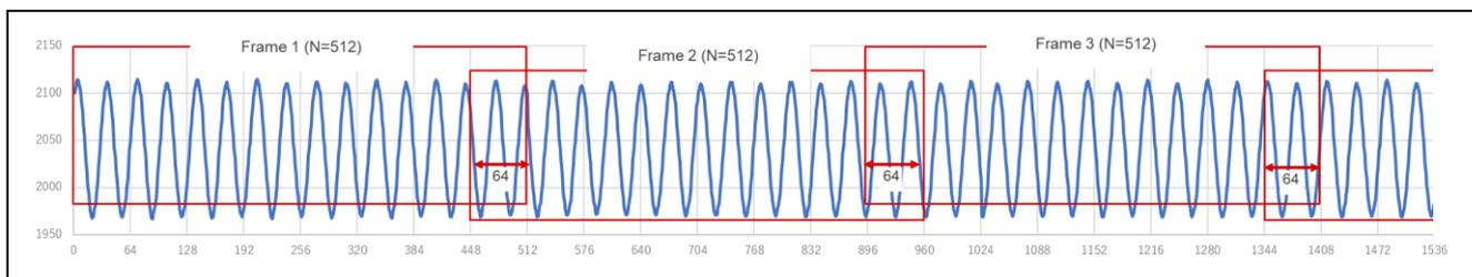
Figure 4-10. A/D Conversion Value of Motor Drive Current
