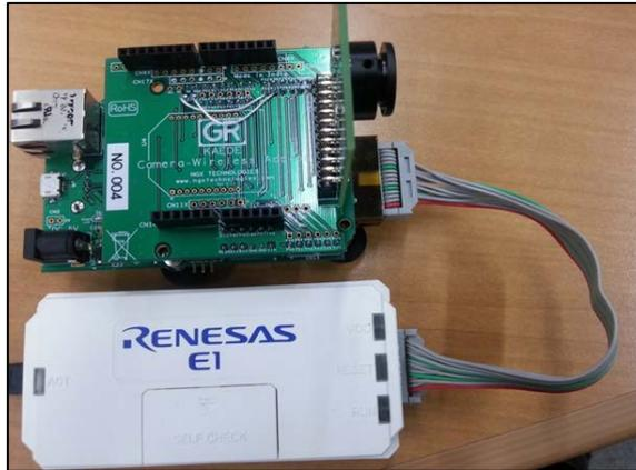
**Figure 12 GR-KAEDE Board (Connected to E1 Emulator)**
