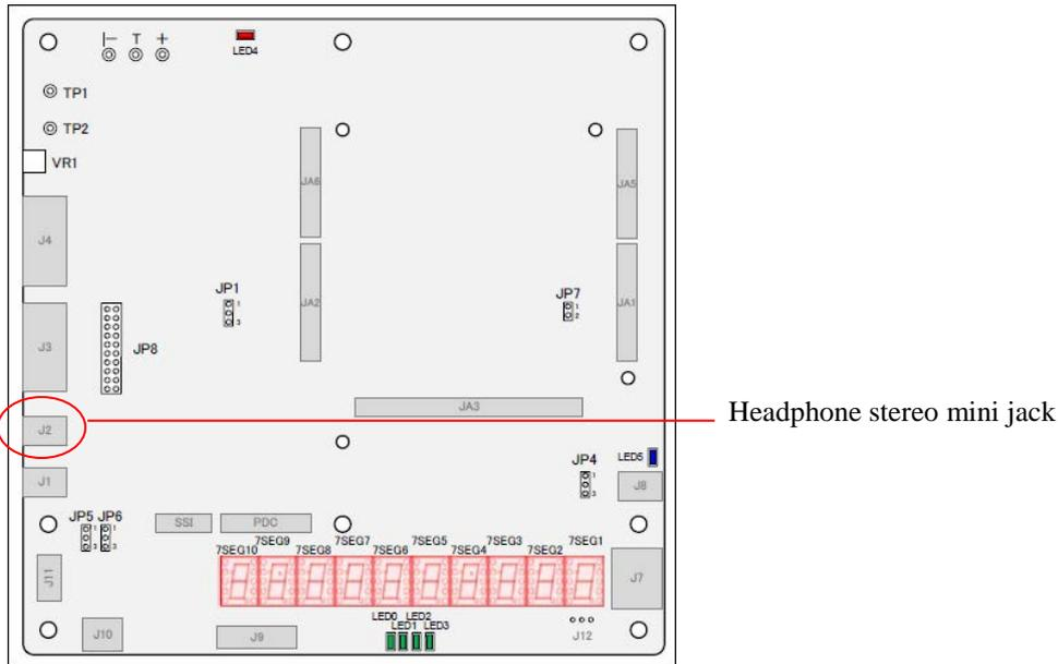
Figure 11 HMI Expansion Board Connector Arrangement Diagram (Headphone Stereo Mini Jack Description)
