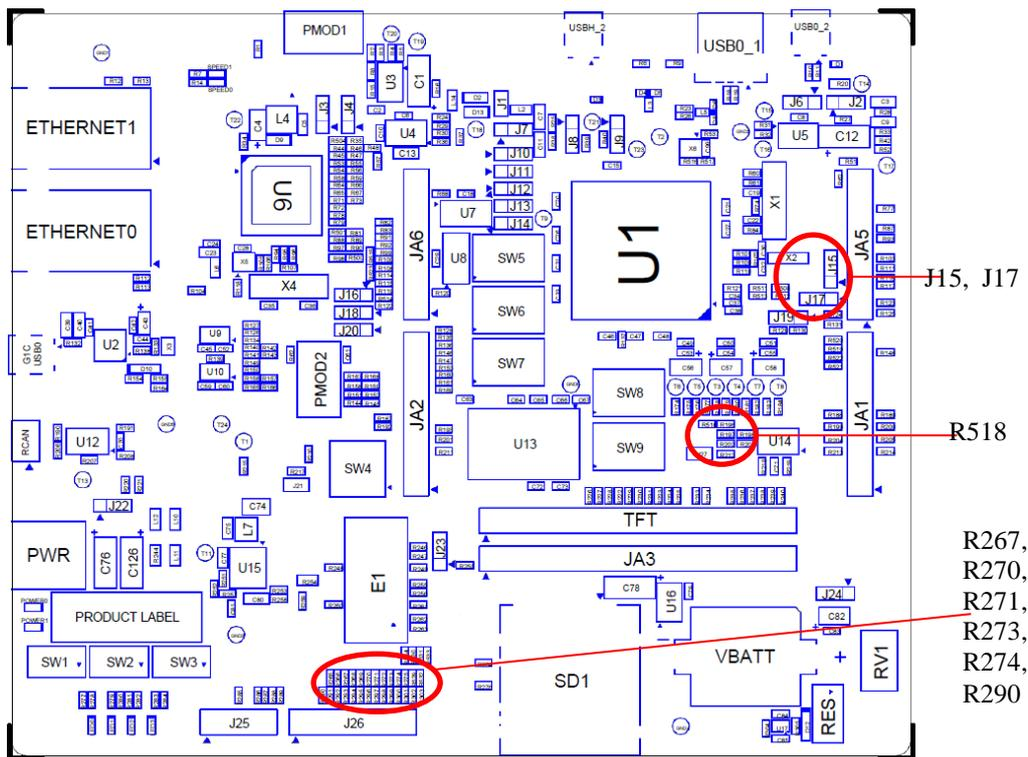
**Figure 4** Locations of Setting Changes (Component Arrangement Diagram: Component Side/Front Side)
