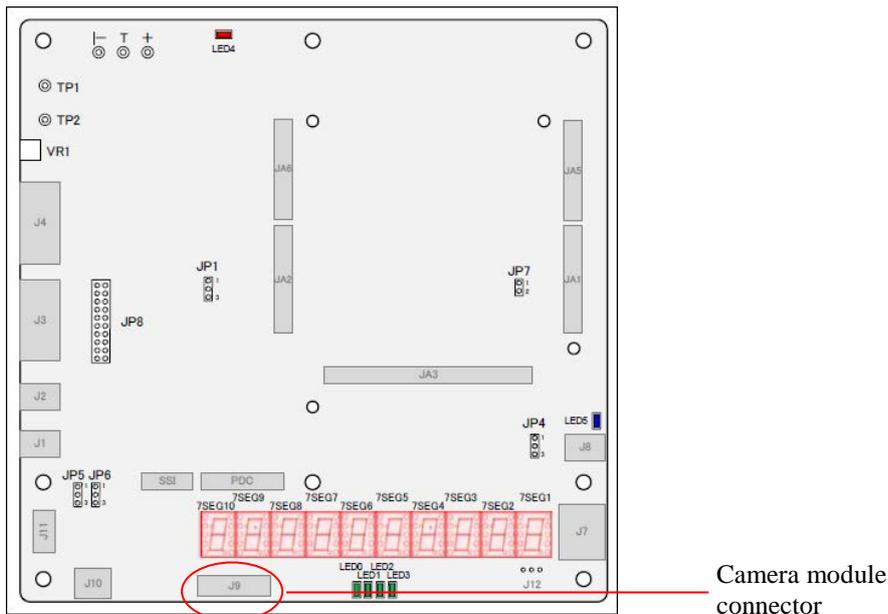
Figure 10 HMI Expansion Board Connector Arrangement Diagram (Camera Module Description)
