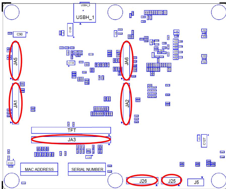
**Figure 3 Connector Attachment Locations (Locations Circled in Red, Component Arrangement Diagram: Solder Side/Back Side)**
