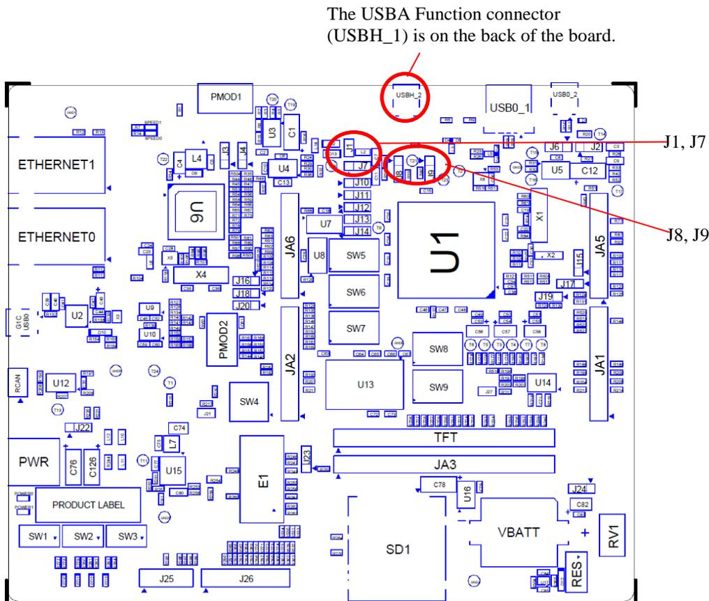
**Figure 8 Jumper Setting Confirmation Locations (Component Arrangement Diagram: Component Side/Front Side)**
