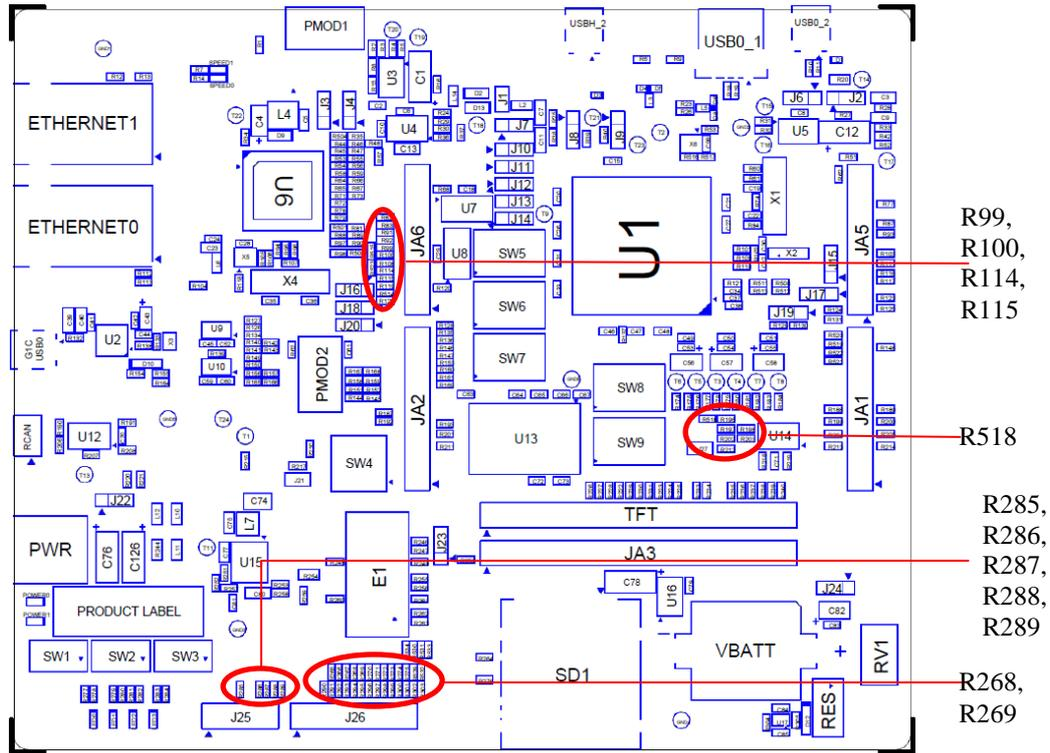
Figure 6 Locations of Setting Changes (Component Arrangement Diagram: Component Side/Front Side)
