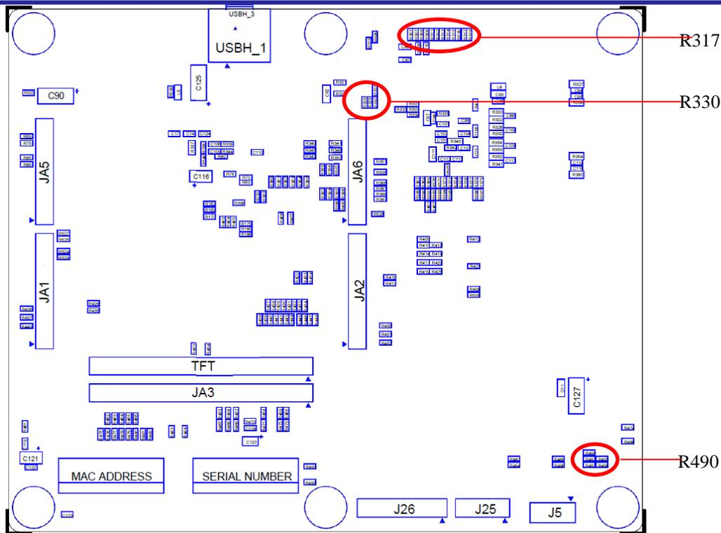
**Figure 5 Locations of Setting Changes (Component Arrangement Diagram: Solder Side/Back Side)**
