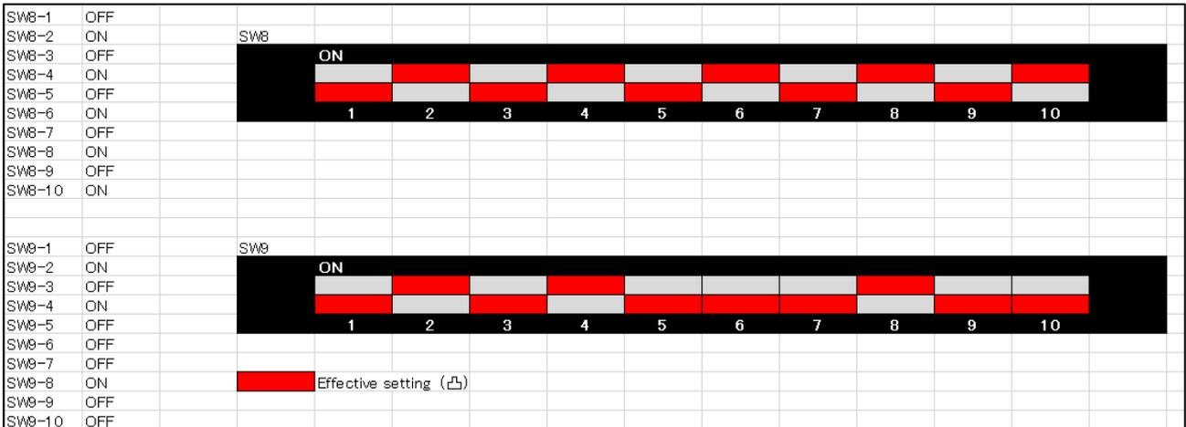
Figure 9 DIP Switch Settings When Using SD Card
