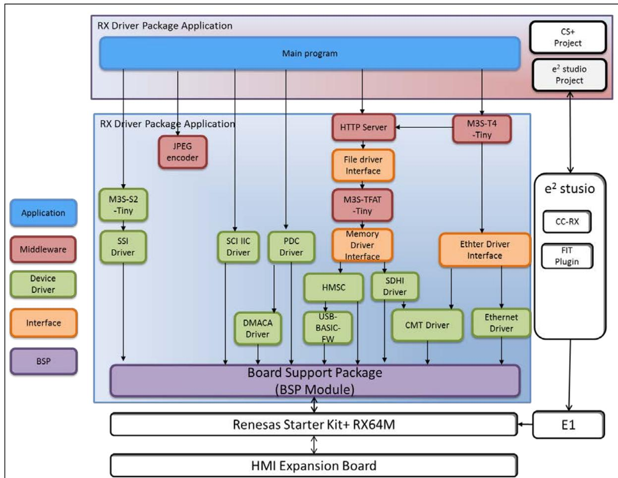
Figure 2 Module Structure
