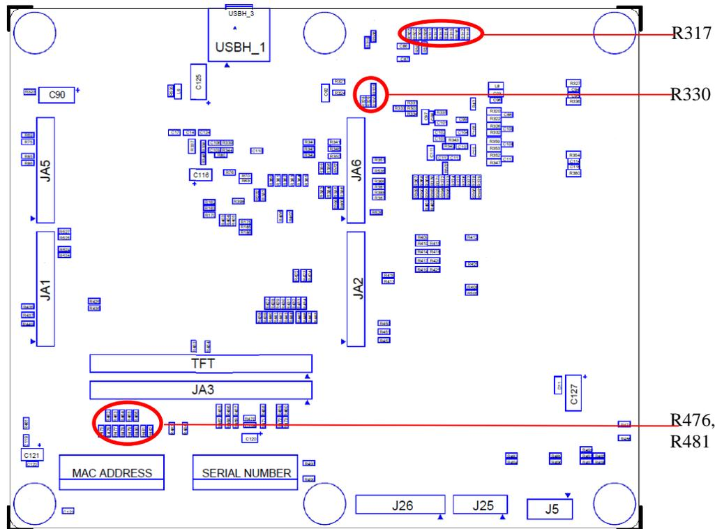
Figure 7 Locations of Setting Changes (Component Arrangement Diagram: Solder Side/Back Side)
