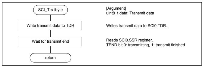
Figure 5.15 1 Byte Data Transmit Function
