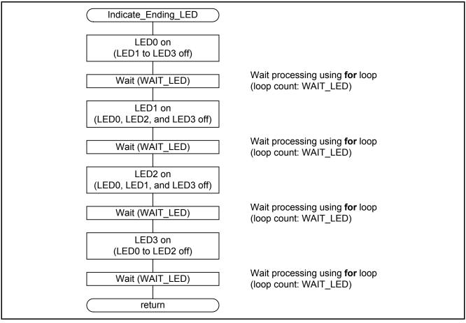
Figure 5.13 Normal Processing Function
