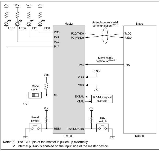
Figure 4.1 Hardware Configuration Diagram of Master Device
