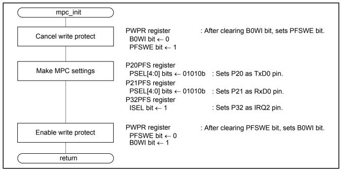
Figure 5.17 MPC Initial Settings Function
