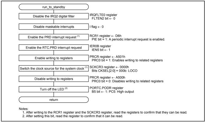
Figure 5.10 Preparation to Enter Software Standby Mode
