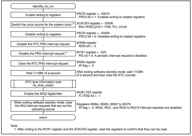
Figure 5.11 Exiting Software Standby Mode
