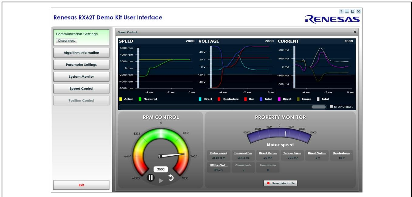
Figure 34 Setting the Speed to Turn the Motor in the GUI Application
