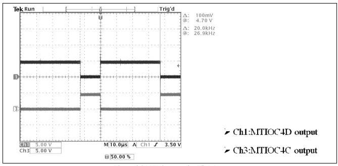
Figure 4-3 MTU3 output for 75% duty
