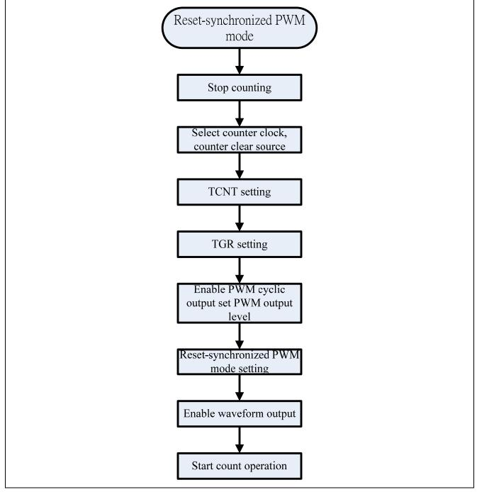
Figure 2-2 Example of Procedure for Setting Reset-Synchronized PWM Mode
