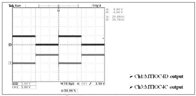
Figure 4-2 MTU3 output for 50% duty
