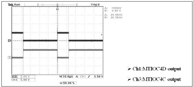
Figure 4-1 MTU3 output for 25% duty
