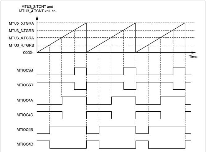
Figure 2-1 Example of Reset-Synchronized PWM mode operation
