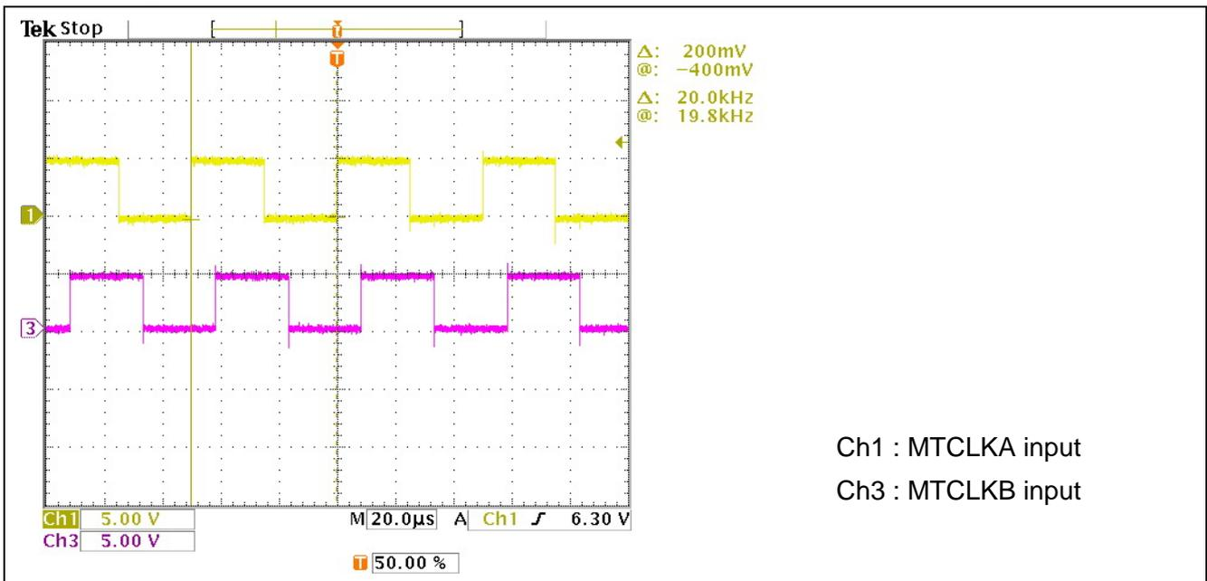
Figure 4-1 MTCLKA and MTCLKB input for encoder pulse
