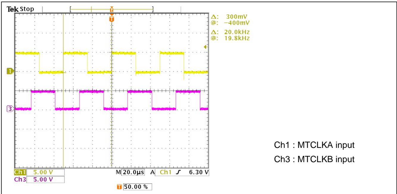
Figure 4-4 MTCLKA and MTCLKB input for encoder pulse
