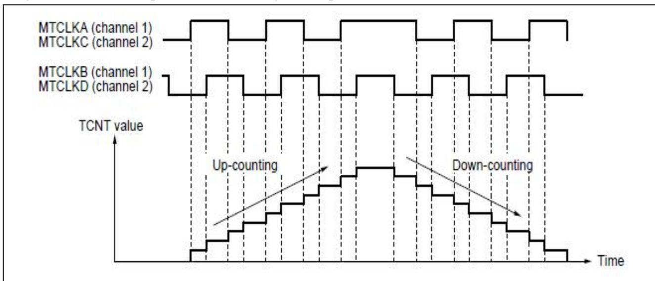
Figure 2-1 Example of Phase Counting Mode operation
