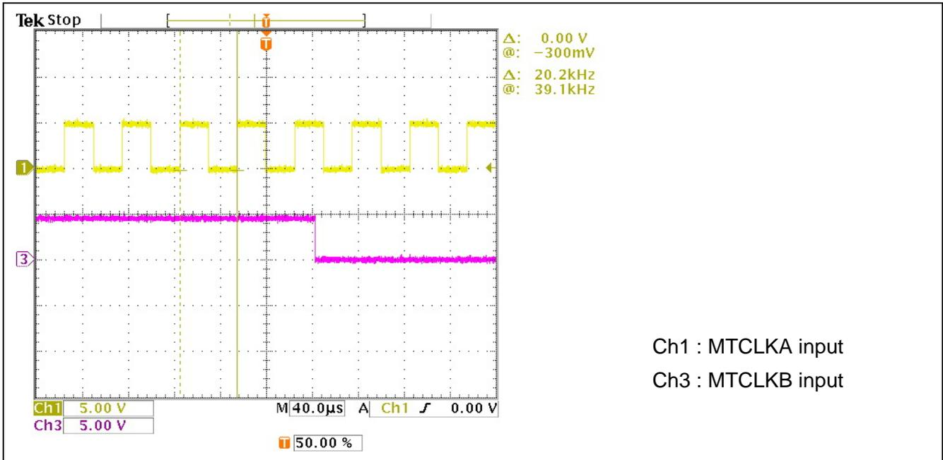
Figure 4-2 MTCLKA and MTCLKB input for encoder pulse
