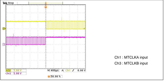
Figure 4-3 MTCLKA and MTCLKB input for encoder pulse
