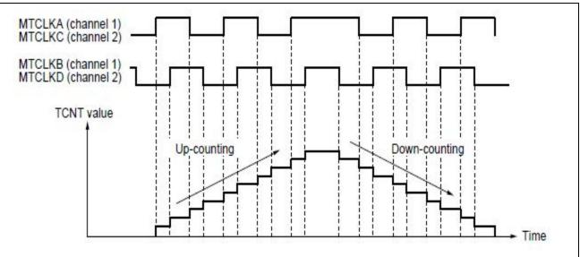
Fig. 2-1 shows an example of Phase Counting Mode operation.
