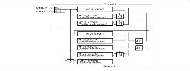
Figure 2-3 Phase Counting Mode Application Example
