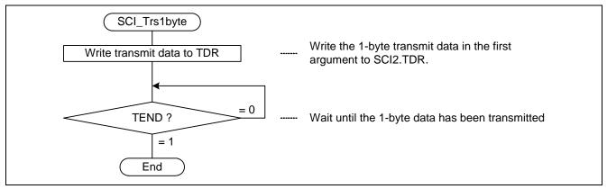
Figure 17 Flowchart (SCI\_Trs1byte) (Master)
