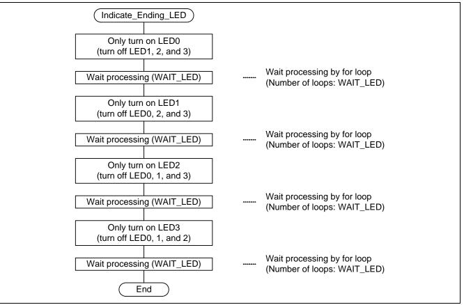
Figure 16 Flowchart (Indicate\_Ending\_LED) (Master)
