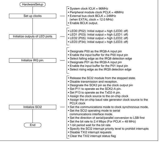
Figure 13 Flowchart (HardwareSetup) (Master)
