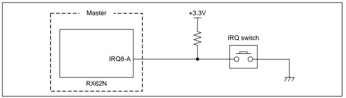
Figure 10 Master IRQ Switch Connection Diagram
