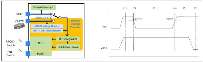
Figure 1.1 Battery Backup Function
