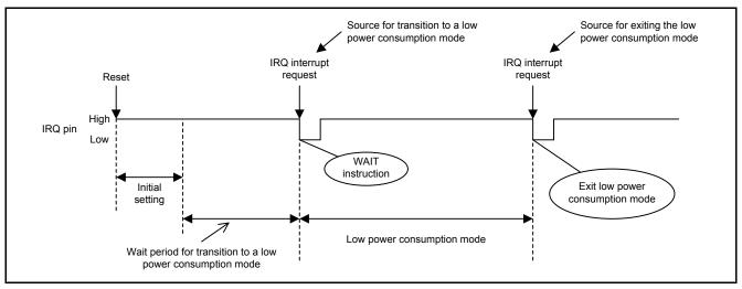
Figure 5.4 Timing for Entering and Exiting a Low Power Consumption Mode Using the IRQ
