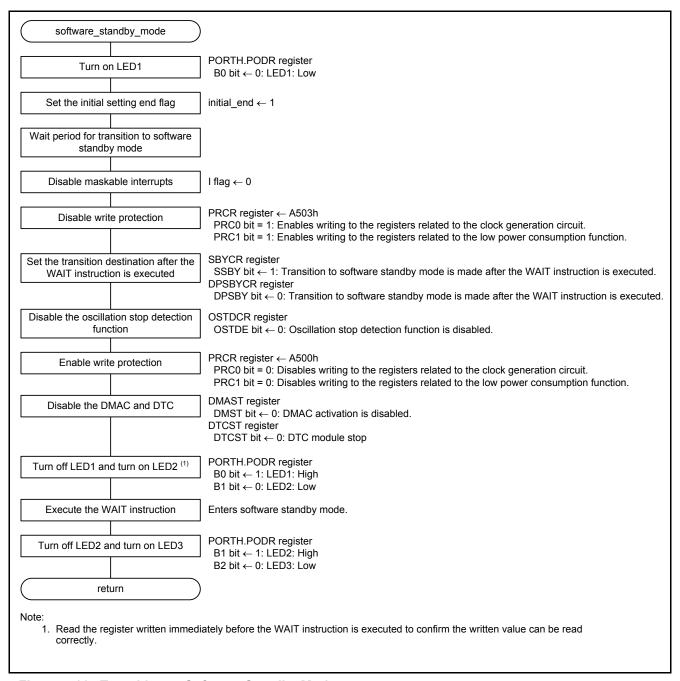
Figure 5.11 Transition to Software Standby Mode
