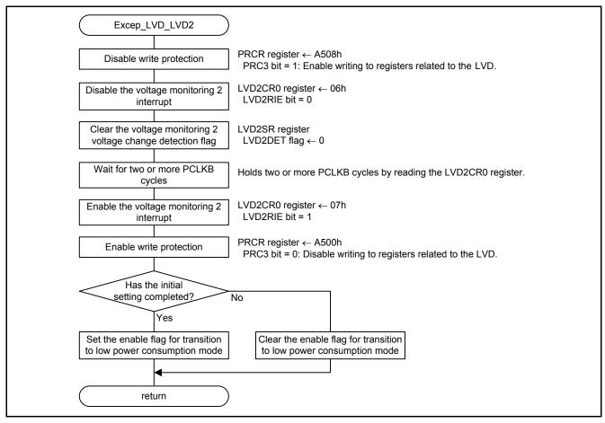
Figure 5.21 LVD2 Interrupt Handling
