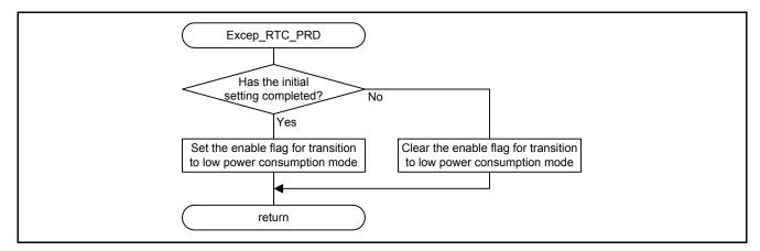
Figure 5.22 RTC.PRD Interrupt Handling
