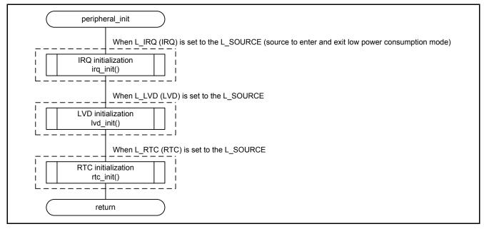
Figure 5.9 Peripheral Function Initialization
