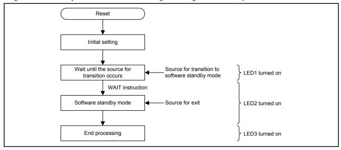
Figure 5.2 Operation Overview when Entering and Exiting Software Standby Mode
