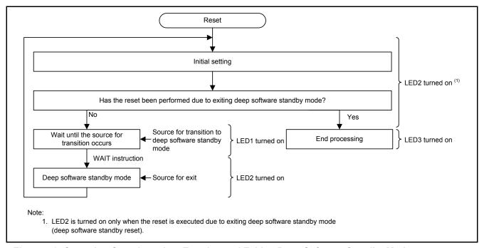
Figure 5.3 Operation Overview when Entering and Exiting Deep Software Standby Mode
