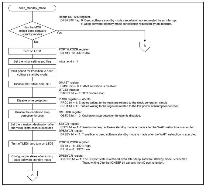
Figure 5.12 Transition to Deep Software Standby Mode (1/3)
