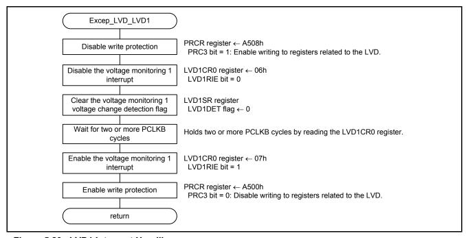
Figure 5.20 LVD1 Interrupt Handling
