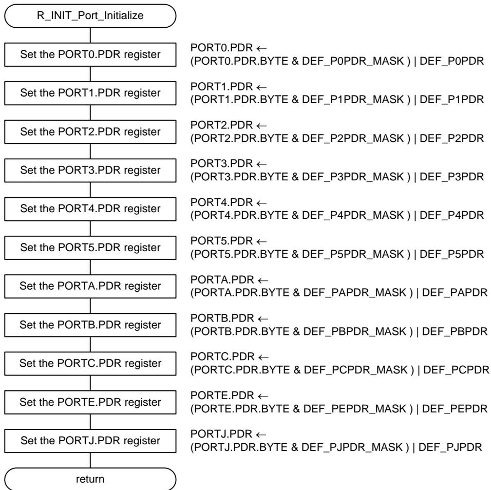
Figure 4.4 Nonexistent Port Initialization
