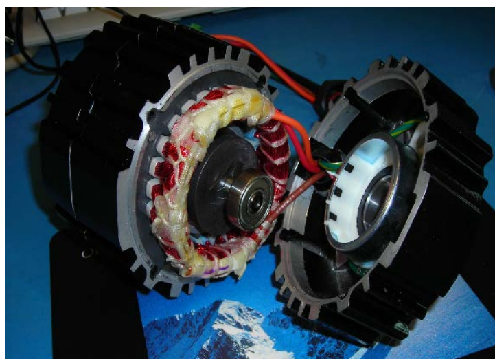
Figure 13 A physical BLDC motor for parameter tuning
