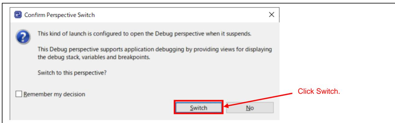
When the load module has been downloaded, the Debug perspective opens. \* The following screenshots illustrate an example configuration for the RX231 group.
