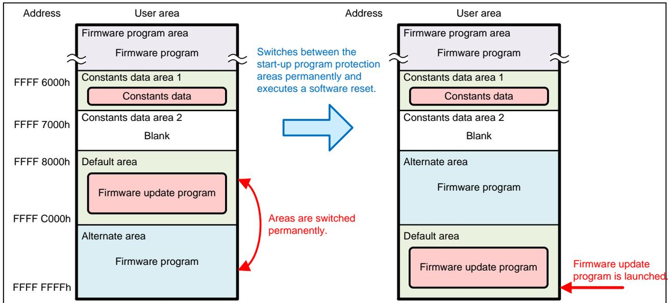
Figure 5.15 Firmware Program Operation (for RX231 Group)
