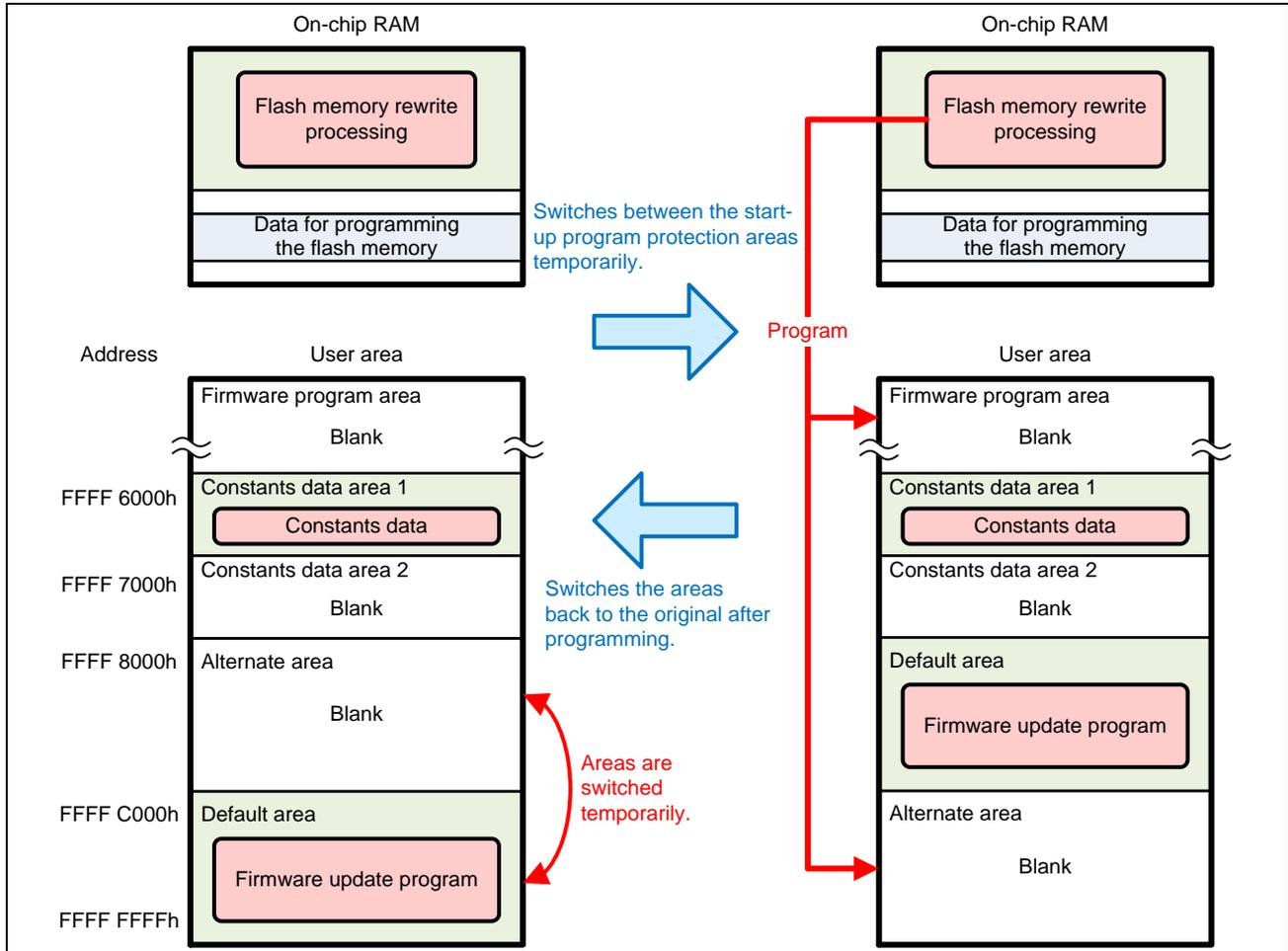
Figure 5.13 Programming the Firmware Program (for RX231 Group)
