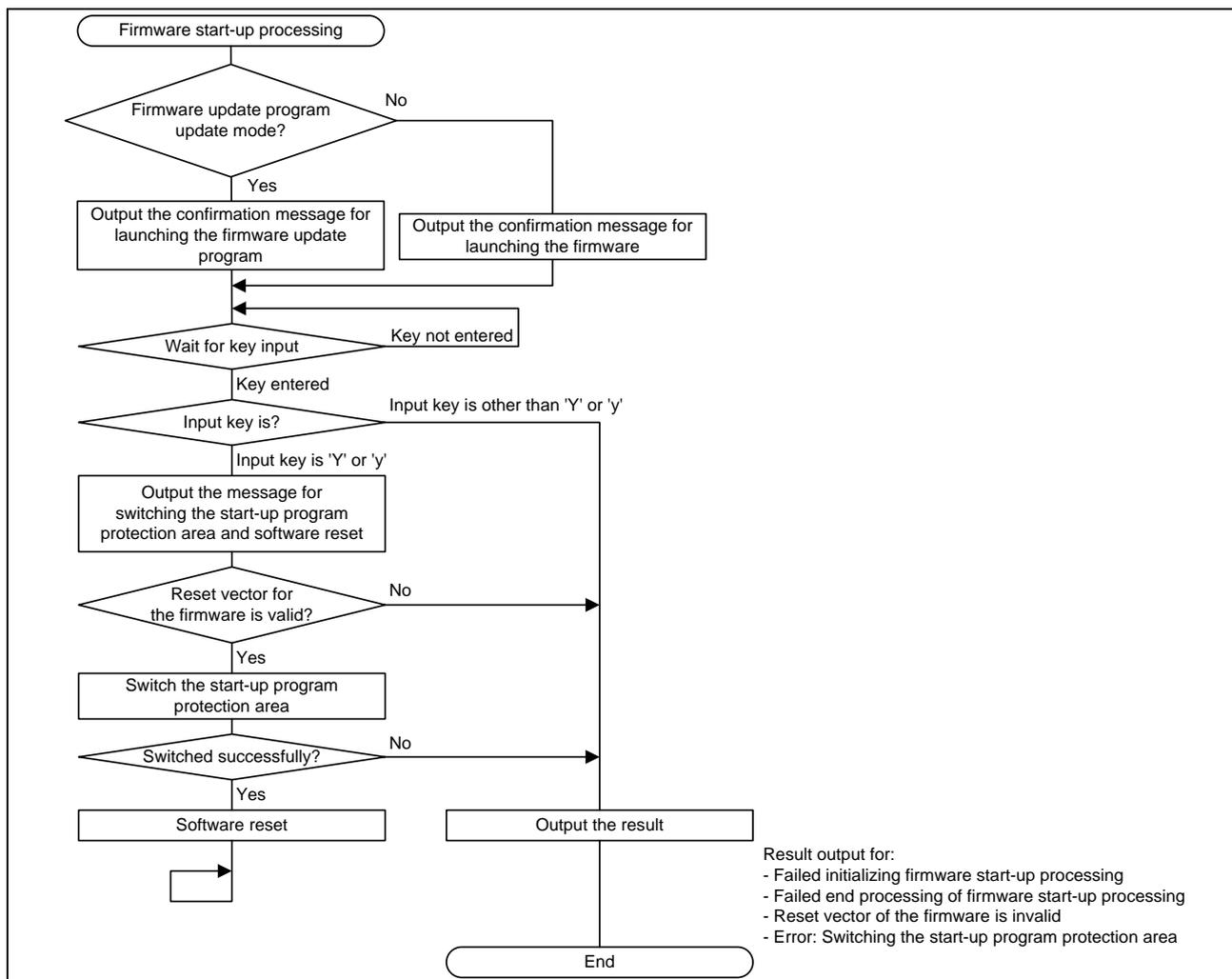
Figure 5.37 Flowchart of Program Start-up Processing
