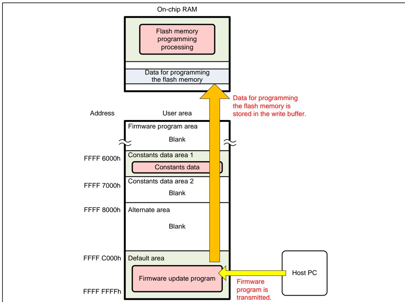
Figure 5.5 Transmitting the Firmware Program (for RX231 Group)
