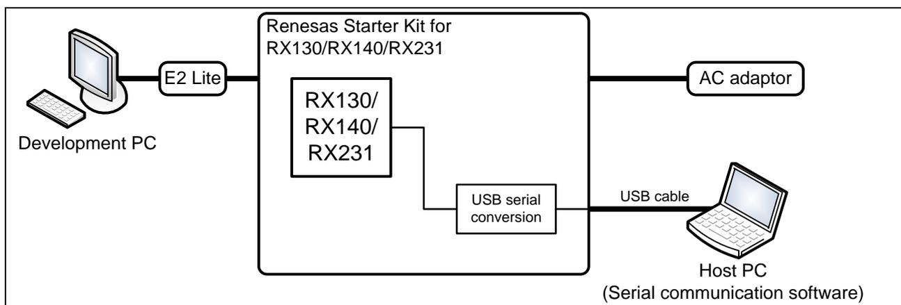
**Figure 4.1 Debug Configuration**
