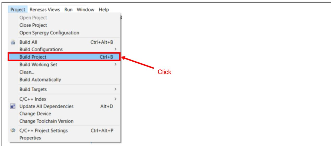
3. The build is completed when the message "Build complete." is displayed in the Console panel.
