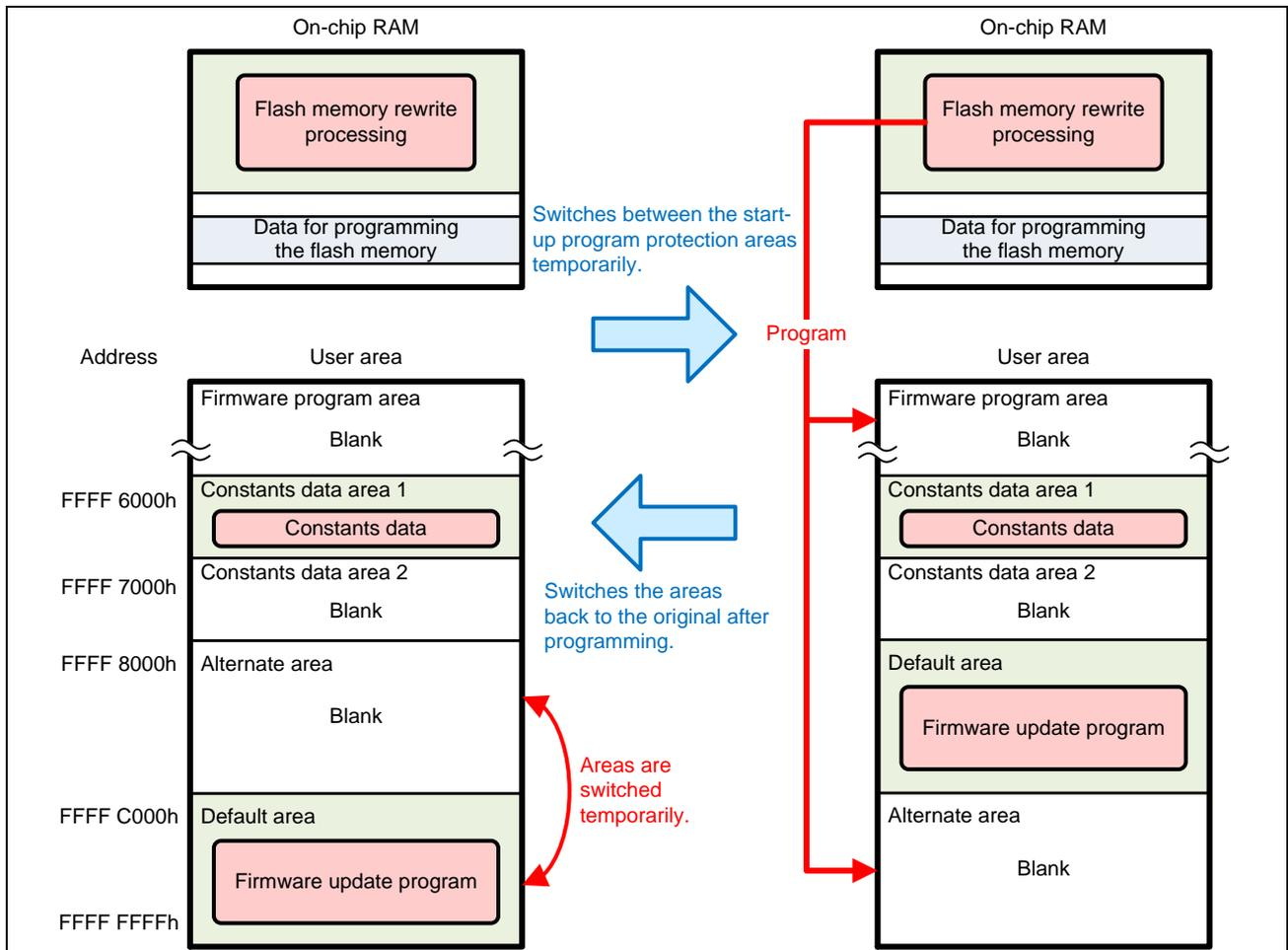
Figure 5.6 Programming the Firmware Program (for RX231 Group)
