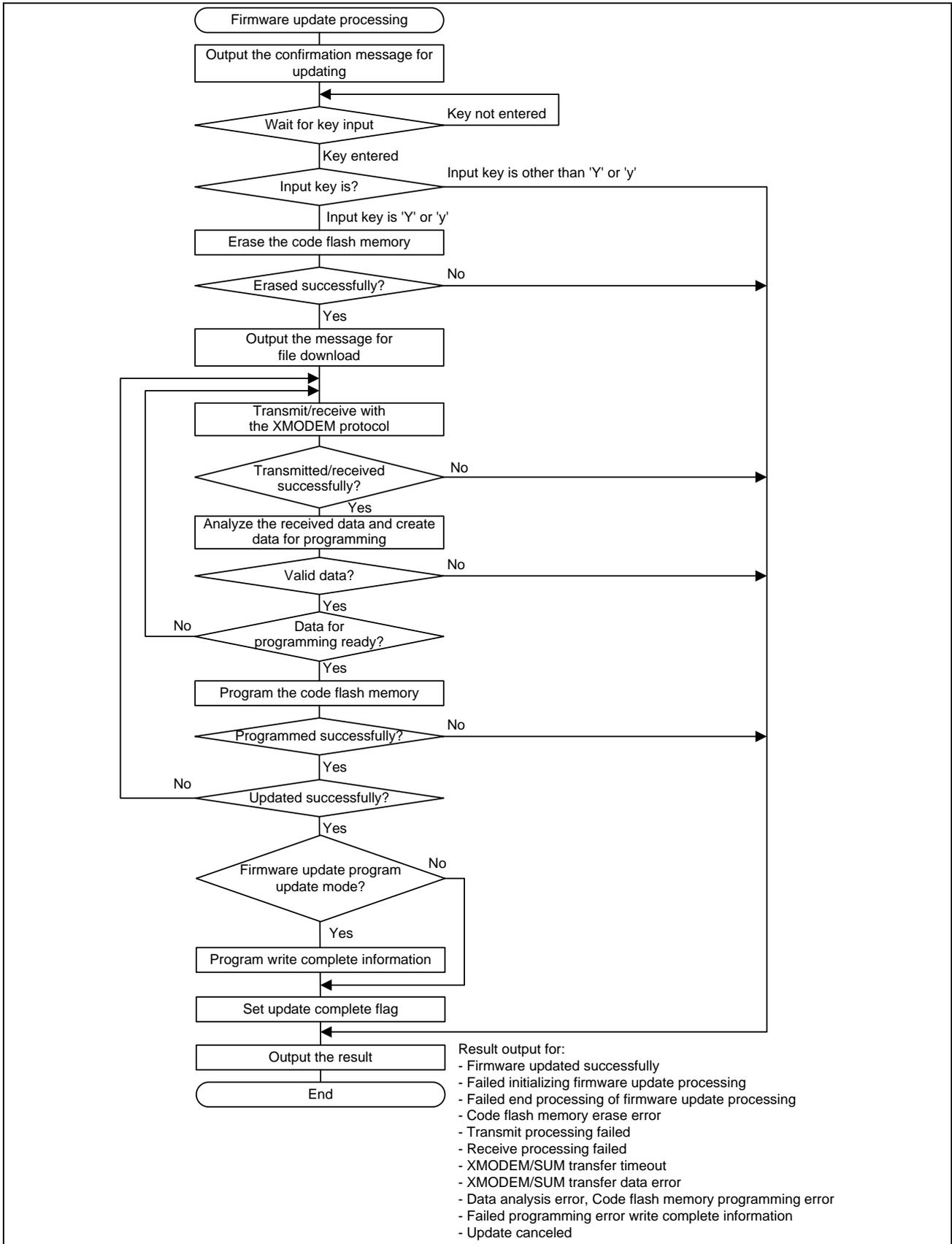
Figure 5.31 Flowchart of Firmware Update Processing
