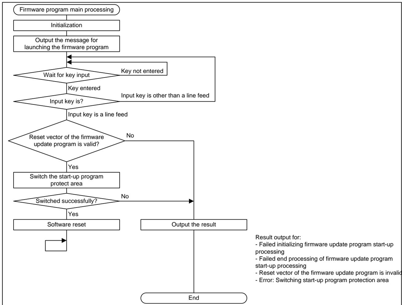
Figure 5.43 Flowchart of the Firmware Program
