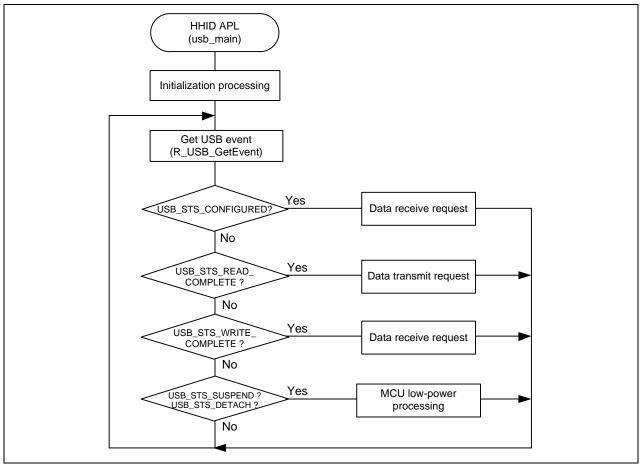
Figure 8-2 Main Loop (Normal mode)
