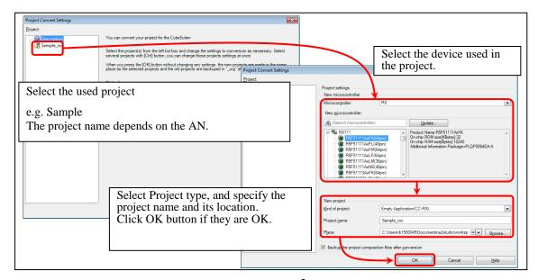
Figure 11-1 Using the e<sup>2</sup> studio project with CS+
