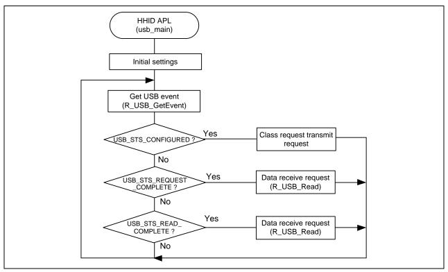
Figure 8-1 Main Loop (Normal mode)
