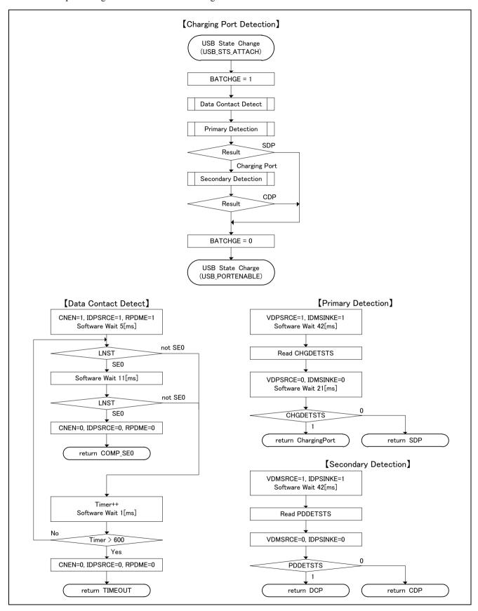
Figure 2-1 PBC processing flow
