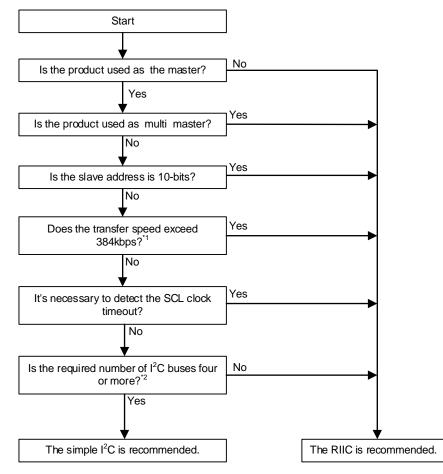
Notes: 1. The transfer speed of RIIC and Simple I<sup>2</sup>C differs depending on the product. 2. The number of RIIC and Simple I<sup>2</sup>C differs depending on the product.
