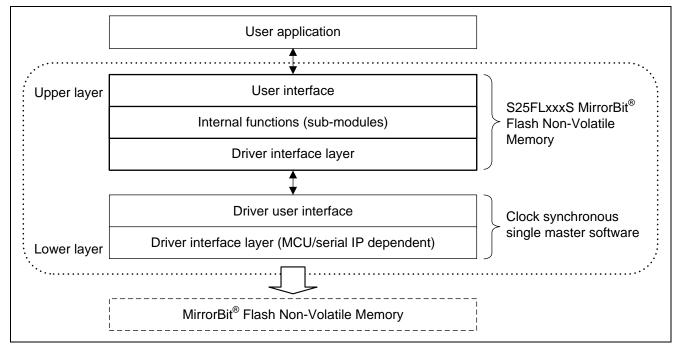
Figure 5.5 Software Configuration
