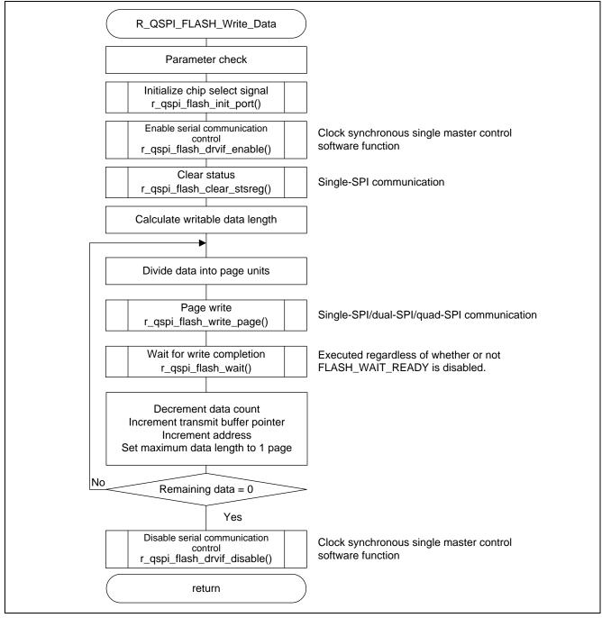
Figure 5.20 Overview of Data Write Processing
