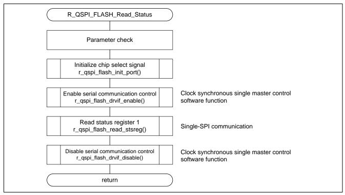
Figure 5.10 Overview of Status Register 1 Read Processing
