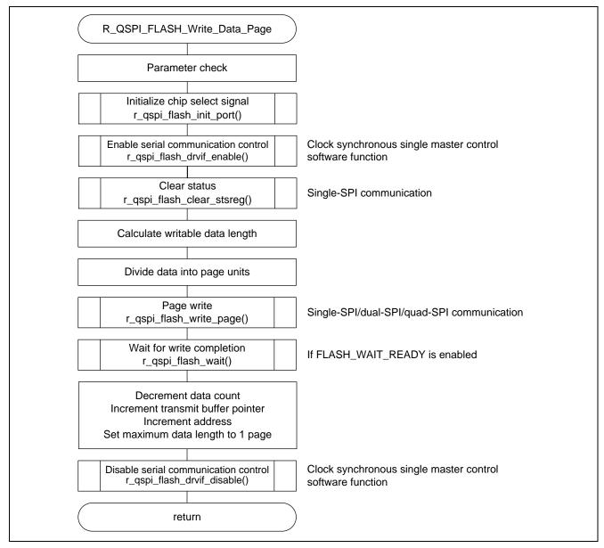
Figure 5.21 Overview of Data Write Processing (for Single-Page Write)
