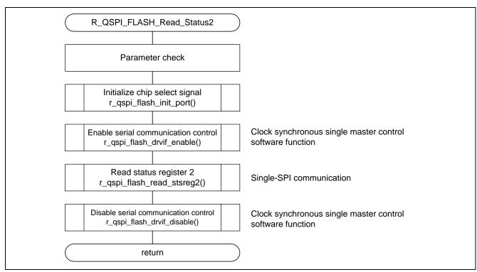
Figure 5.11 Overview of Status Register 2 Read Processing
