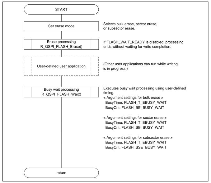
Figure 5.24 Using R\_QSPI\_FLASH\_Wait() to Wait for Erase Processing Completion
