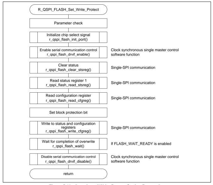
Figure 5.12 Overview of Write Protect Setting Processing
