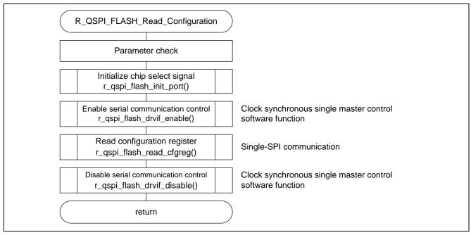
Figure 5.14 Overview of Configuration Register Read Processing
