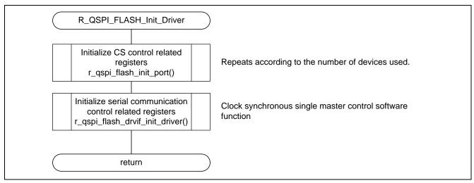
Figure 5.8 Overview of Driver Initialization Processing
