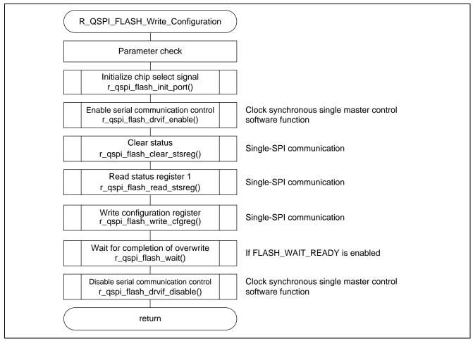
Figure 5.15 Overview of Configuration Register Write Processing
