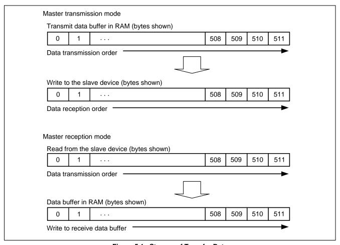
Figure 5.1 Storage of Transfer Data
