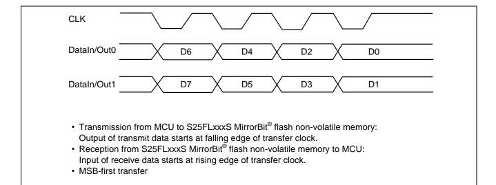
Figure 5.3 Dual-SPI Clock Synchronous Mode Timing Settings
