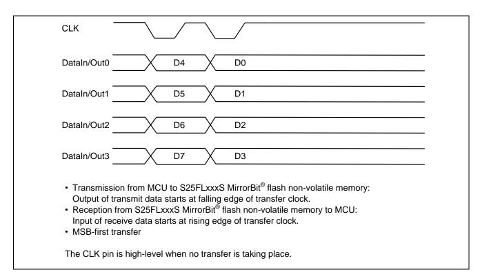
Figure 5.4 Quad-SPI Clock Synchronous Mode Timing Settings
