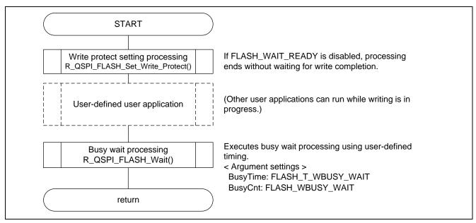
Figure 5.13 OUsing R\_QSPI\_FLASH\_Wait() to Wait for Write Protect Setting Completion
