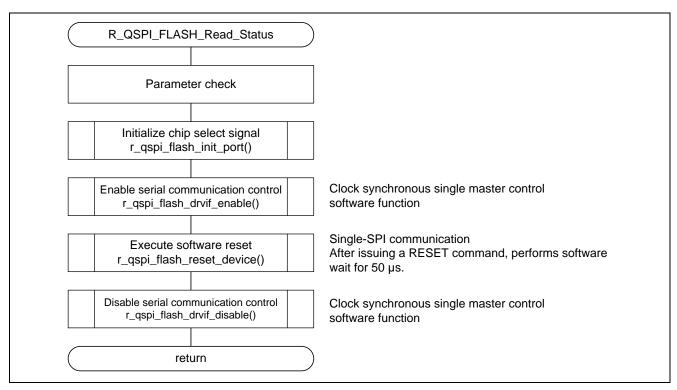
Figure 5.9 Overview of Device Initialization Processing
