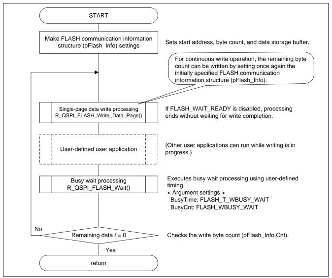
Figure 5.22 Using R\_QSPI\_FLASH\_Wait() to Wait for Data Write Processing (for Single-Page Write)
