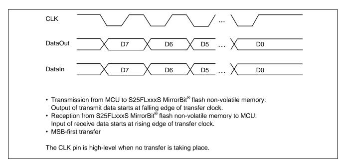
Figure 5.2 Single-SPI Clock Synchronous Mode Timing Settings
