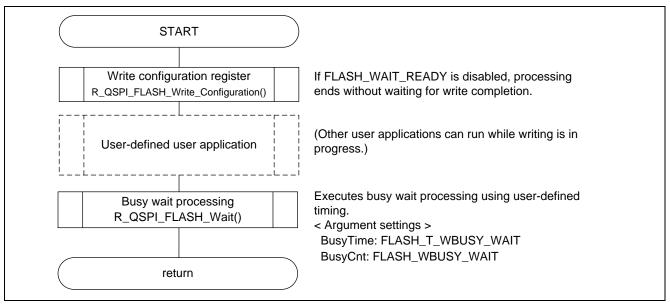
Figure 5.16 Using R\_QSPI\_FLASH\_Wait() to Wait for Write Protect Setting Completion
