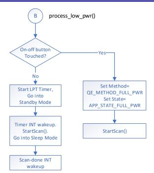
When the system is running in *application state low power*, the MCU goes in and out of low power modes as it periodically needs to start scans and check for button touches. When this function is called, the MCU is temporarily awake due to a scan-done interrupt. There is no user-specific code present in this function.
