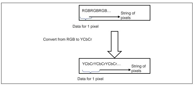
Figure 1 Placement of RGB and YCbCr Data in Memory
