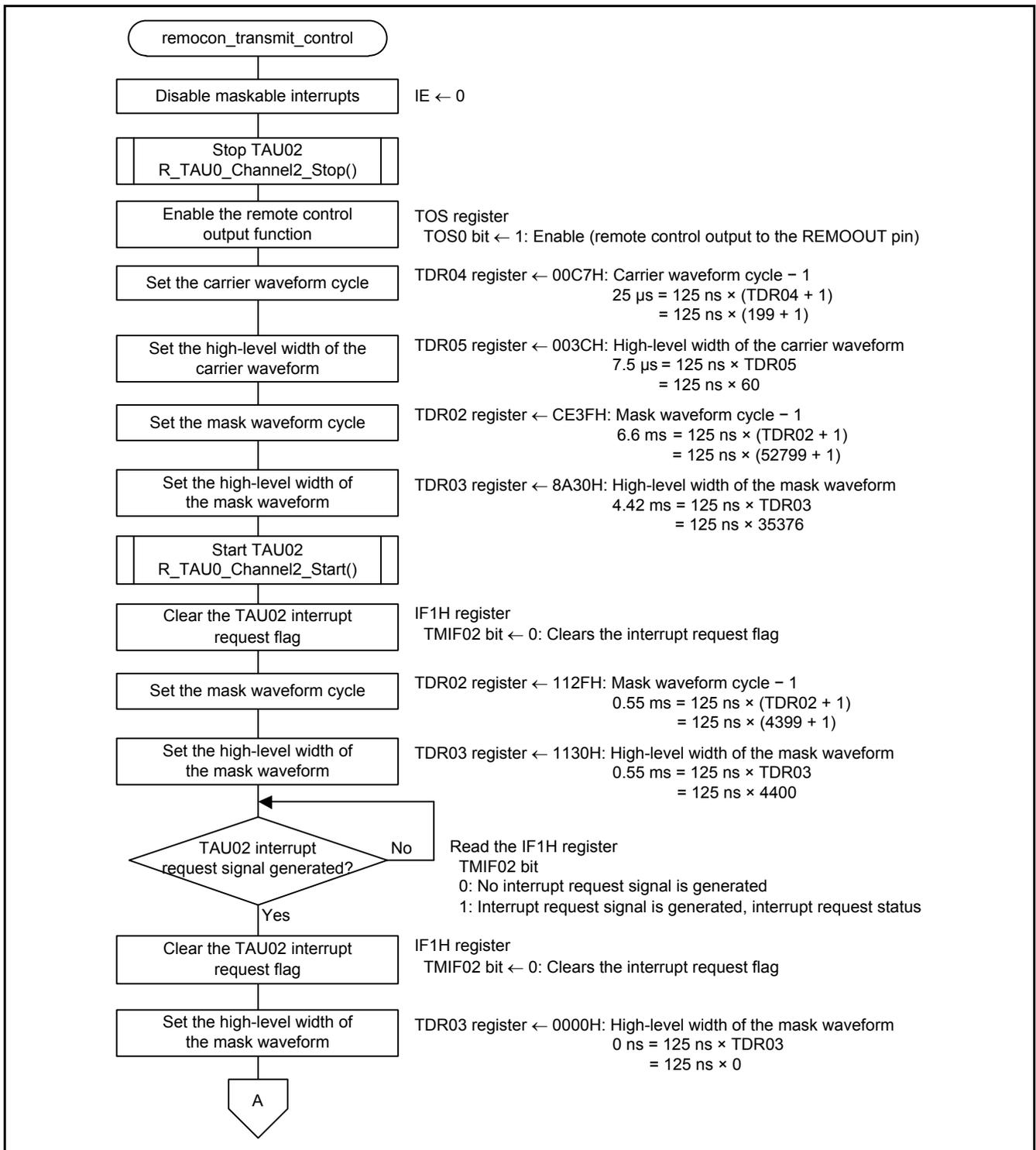
Figure 4.14 Remote Control Output Control Setting (1/2)
