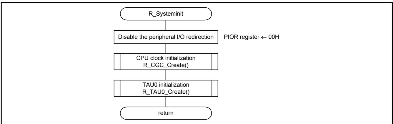
Figure 4.4 Peripheral Function Initialization
