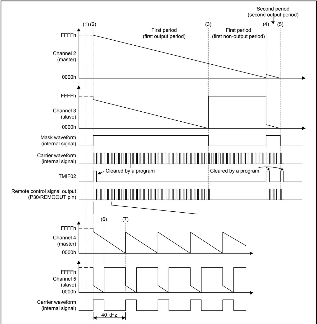
Figure 4.1 Behavior of Remote Control Output
