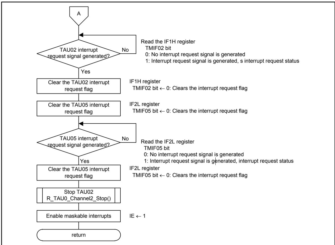
Figure 4.15 Remote Control Output Control Setting (2/2)
