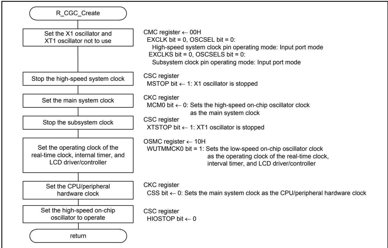
Figure 4.5 CPU Clock Initialization
