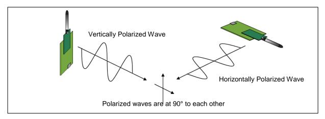
Figure 3-2 Antenna polarization
