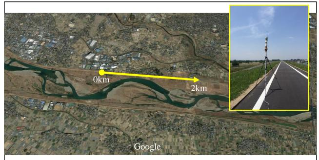
[Measurement condition] CH=30(926.7MHz), Output Power=+13dBm(20mW)
