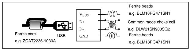
Figure 3-5 Example of USB noise suppression
