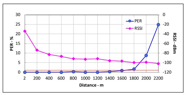
Figure 4-2 Packet error rate in each measurement point
