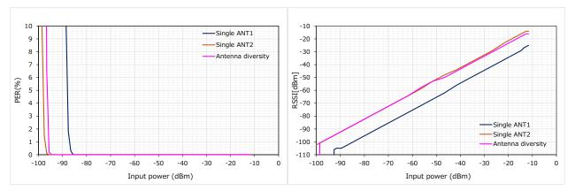
Figure 6. PER (ATT10dB on ANT1 side)
