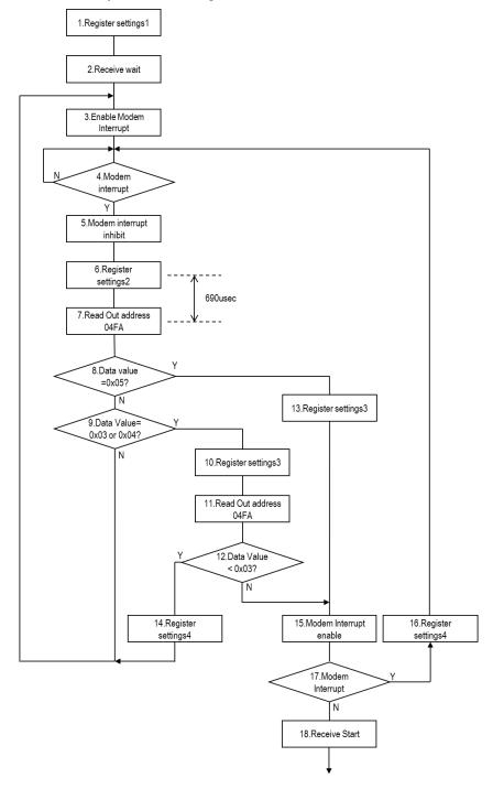
Figure 1. Flowchart for G1H/RAA604S00 based antenna diversity
