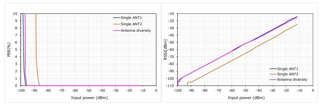
Figure 4. PER (ATT10dB on ANT2 side)
