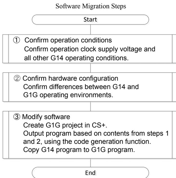
For a detailed example, refer to RL78/G14 Timer RD (Reset Synchronized PWM Mode) CC-RL (document R01AN2506EJ0100, referred to as RL78/G14 Application Note, herein). The Application Note explains how to modify the G1G program with the G14 program. RL78/G1G hardware is configured to support the RL78/G1G target board (YQB-R5F11EFA-TB) CPU board mounted on R5F11EFA.
