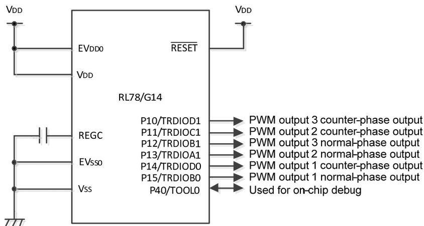
From G14 Application Note: Figure 3.1 Hardware Configuration
