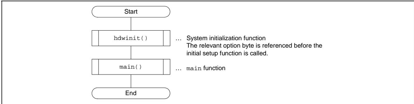
Figure 6.2 Overview of Processing Flow
