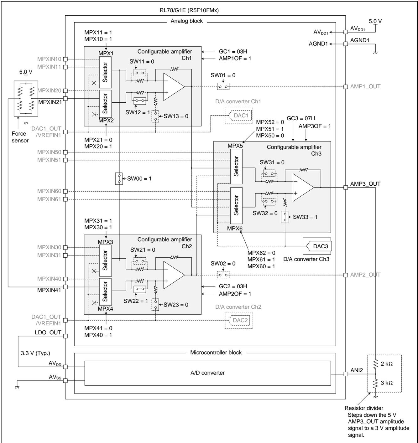
**Figure 5.3 Connection Between Configurable Amplifier Channels Ch1 to Ch3 and Force Sensor, and Between Configurable Amplifier Channels Ch1 to Ch3 and A/D Converter**
