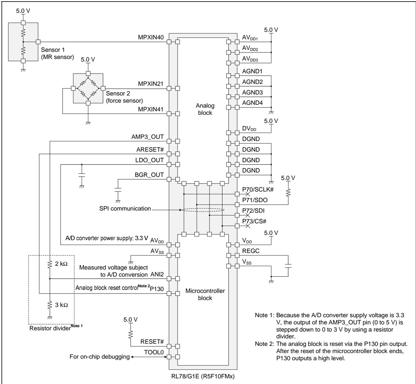
Figure 4.1 Hardware Configuration
