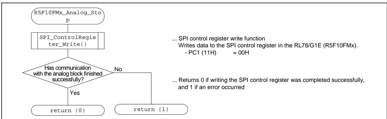
Figure 6.13 Flowchart for R5F10FMx\_Analog\_Stop Function
