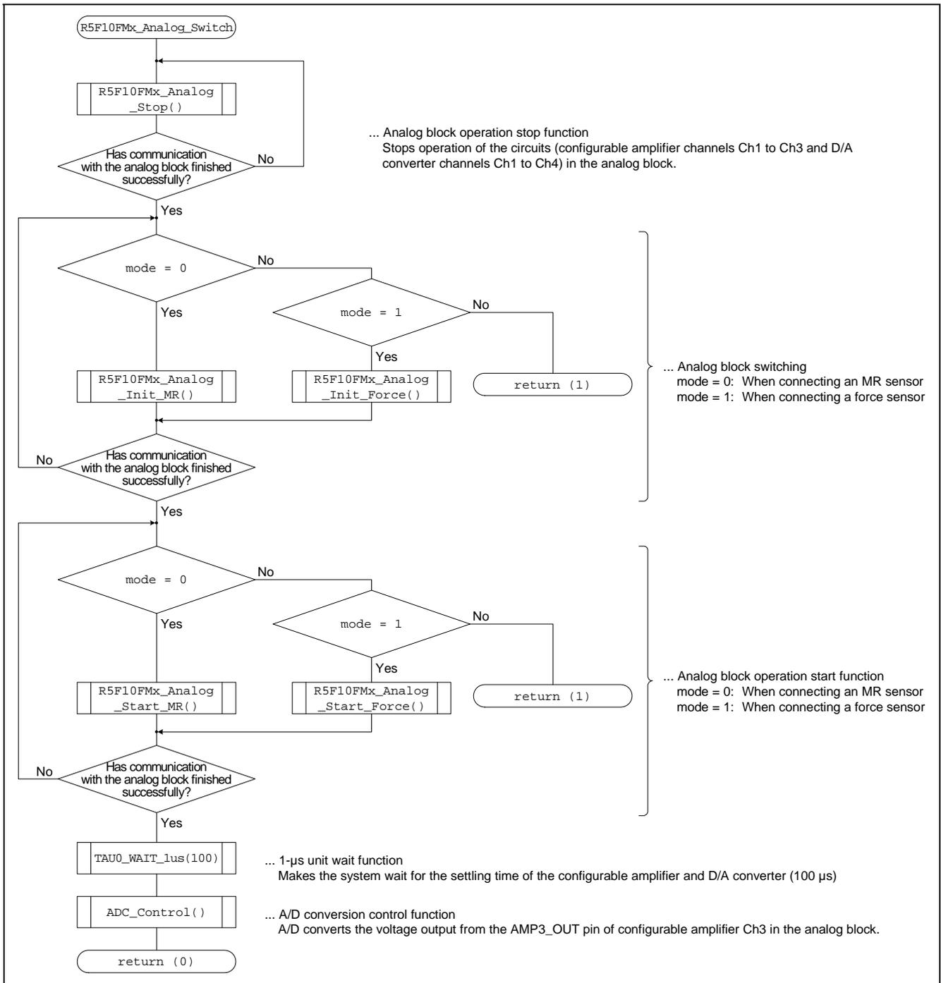
Figure 6.8 Flowchart for R5F10FMx\_Analog\_Switch Function
