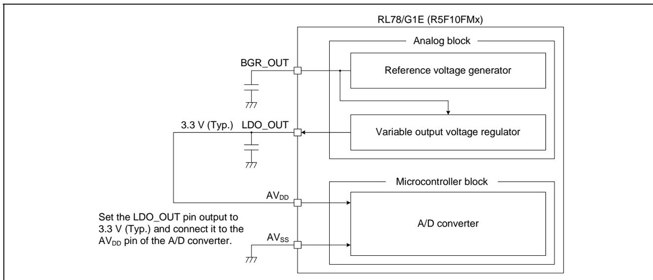
**Figure 5.1 Connection Between Variable Output Voltage Regulator and A/D Converter**
