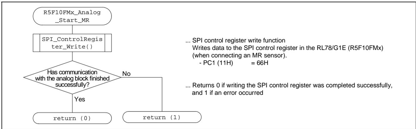
Figure 6.11 Flowchart for R5F10FMx\_Analog\_Start\_MR Function
