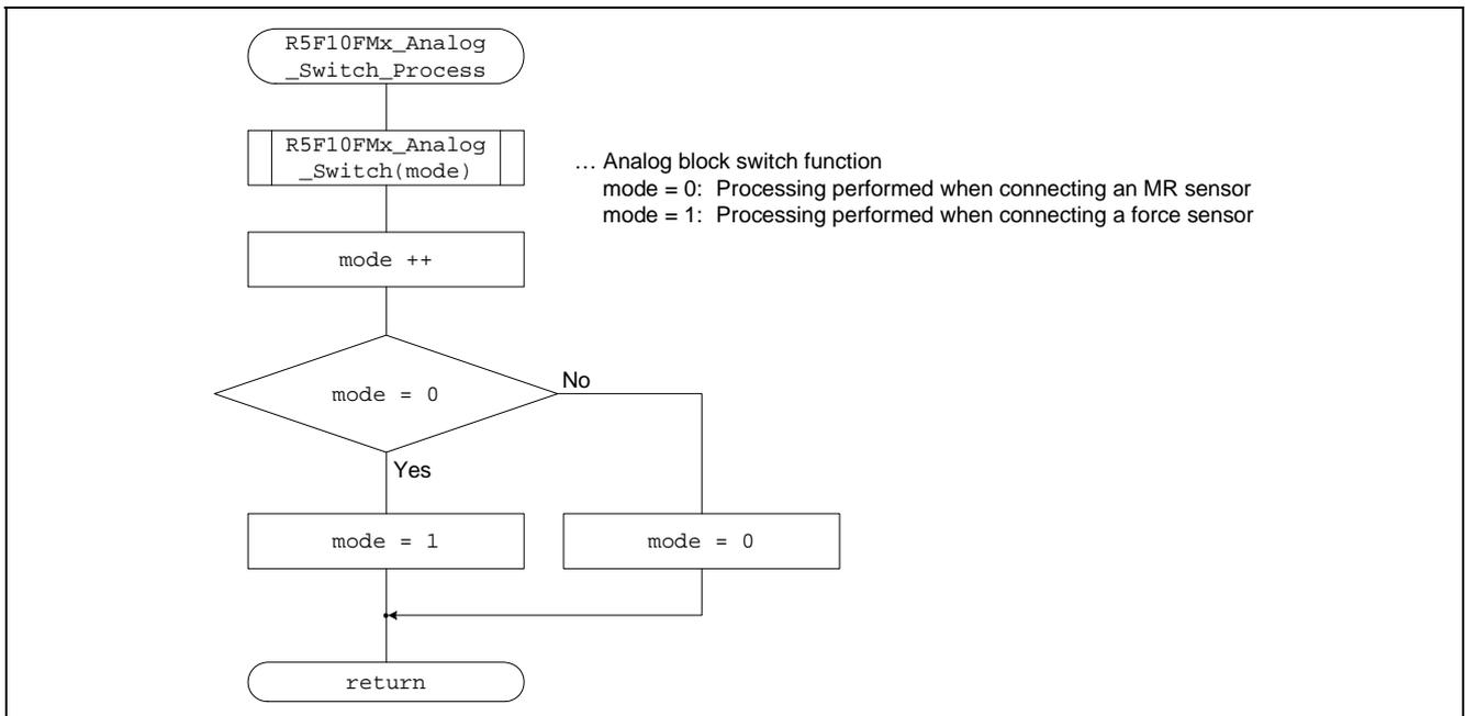
Figure 6.7 Flowchart for R5F10FMx\_Analog\_Switch\_Process Function
