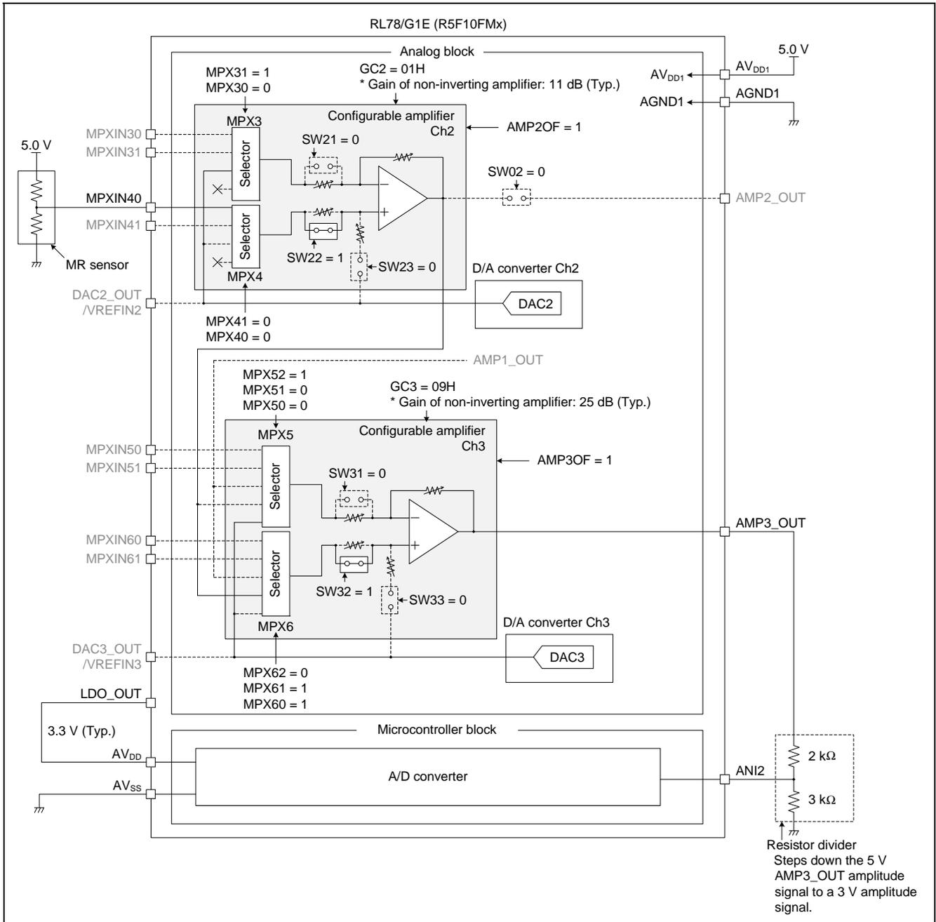
Figure 5.2 Connection Between Configurable Amplifier Channels Ch2 and Ch3 and MR Sensor, and Between Configurable Amplifier Channels Ch2 and Ch3 and A/D Converter
