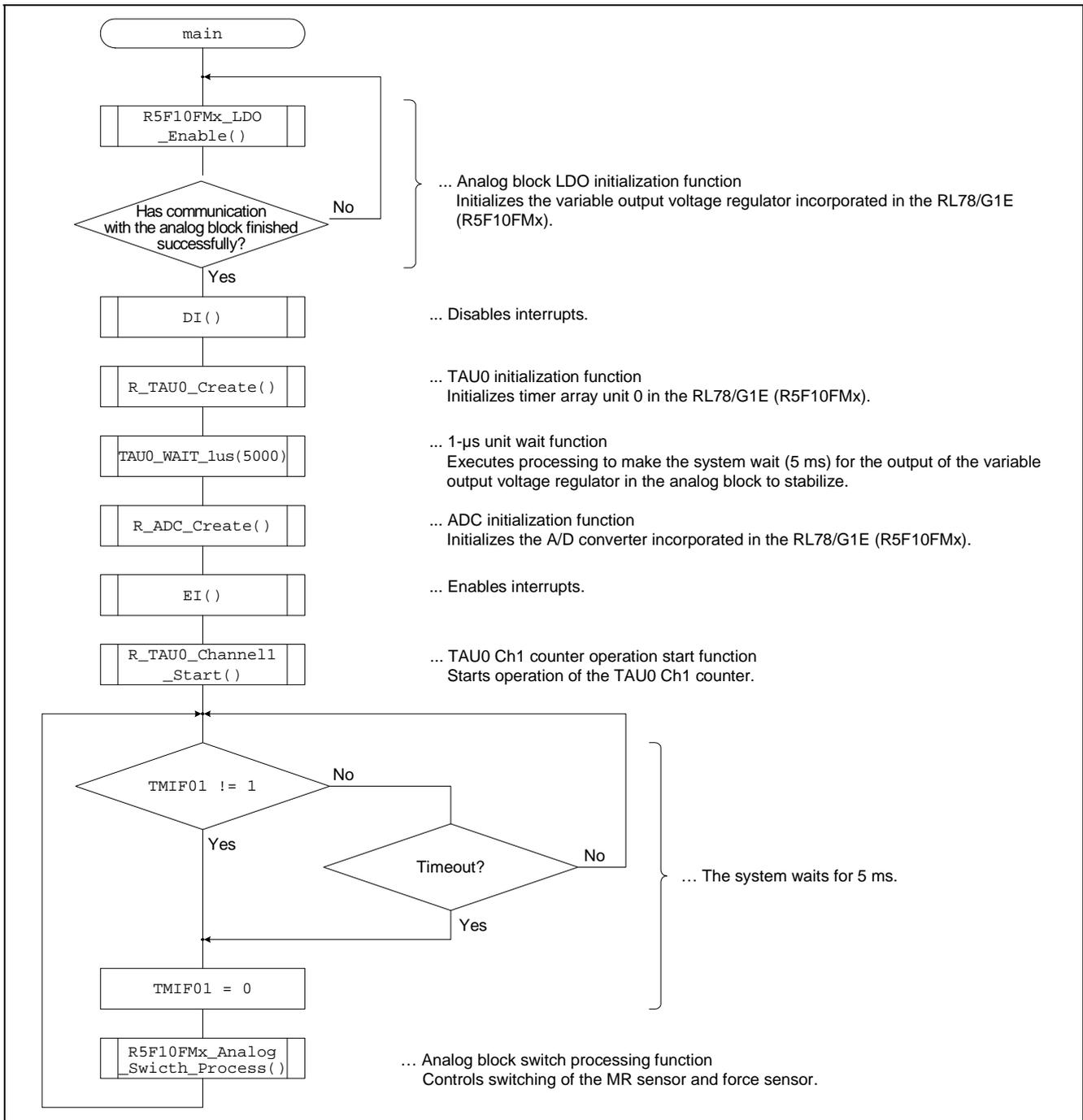
Figure 6.5 Flowchart for main Function
