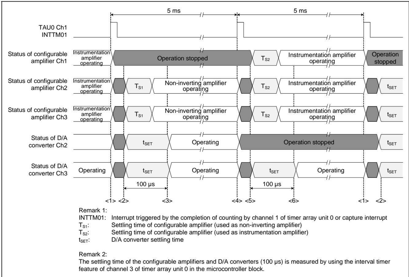
**Figure 6.1 Timing of Amplifier Reconfiguration in Analog Block**
