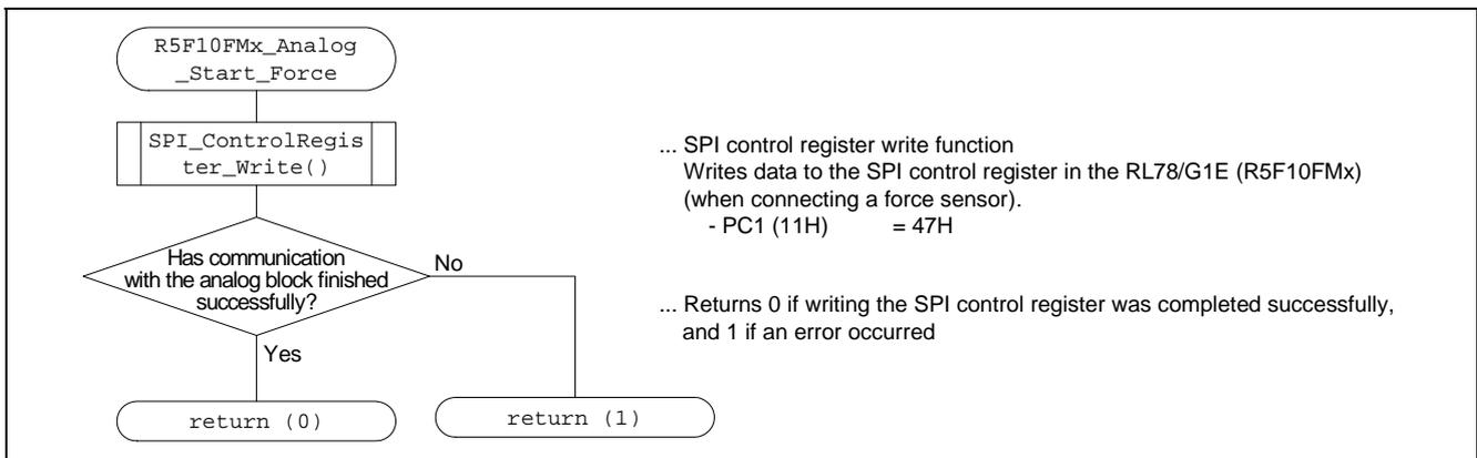
Figure 6.12 Flowchart for R5F10FMx\_Analog\_Start\_Force Function
