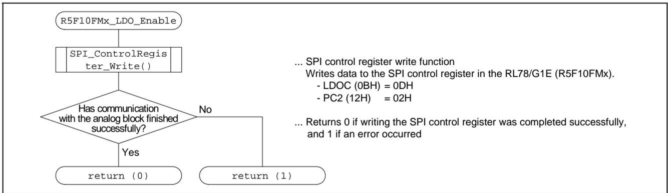
Figure 6.6 Flowchart for R5F10FMx\_LDO\_Enable Function
