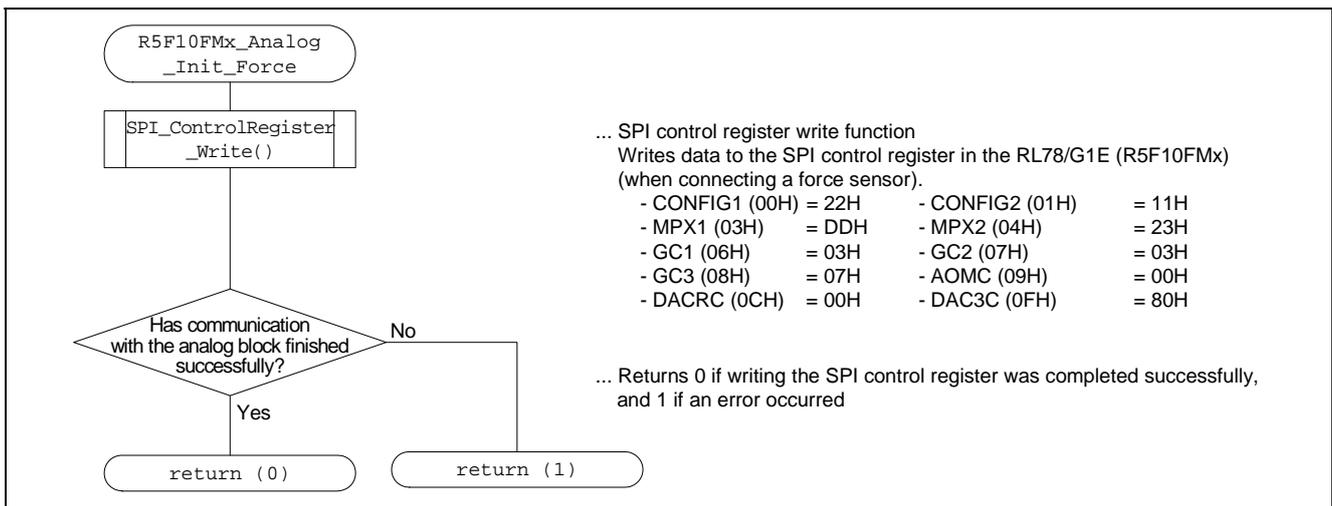
Figure 6.10 Flowchart for R5F10FMx\_Analog\_Init\_Force Function
