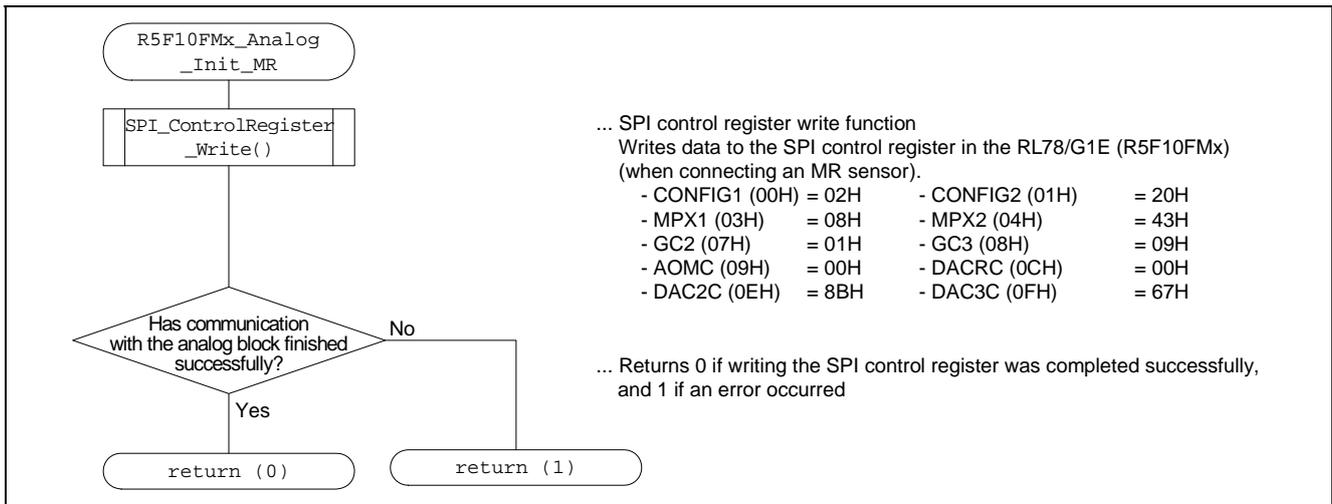
Figure 6.9 Flowchart for R5F10FMx\_Analog\_Init\_MR Function
