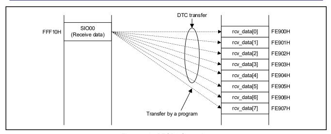
Figure 4.3 DTCD0 Operation
