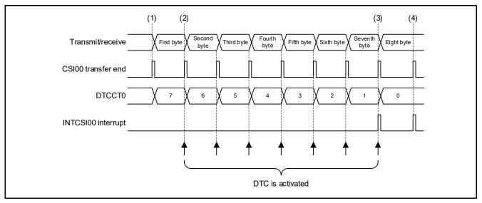
Figure 4.2 Timing of Transmission/Reception and DTC Activation
