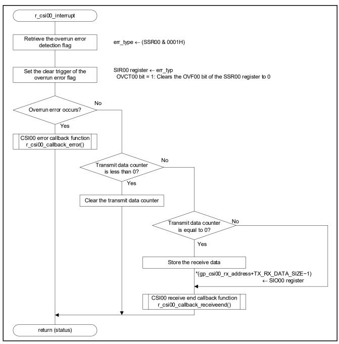
Figure 4.13 CSI00 Transfer End Interrupt
