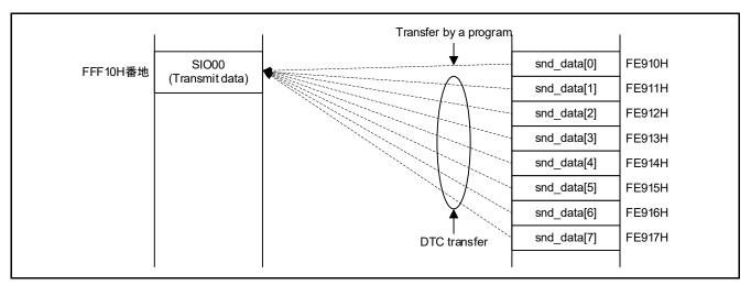
Figure 4.4 DTCD1 Operation
