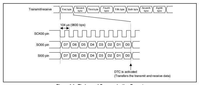
Figure 1.1 Timing and Communication Format
