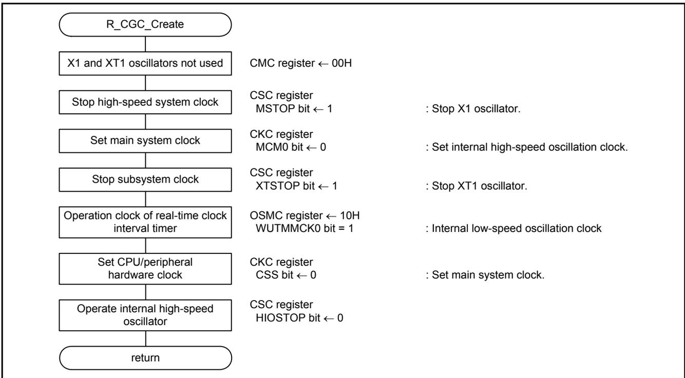
Figure 4.6 Initial Setting of the CPU
