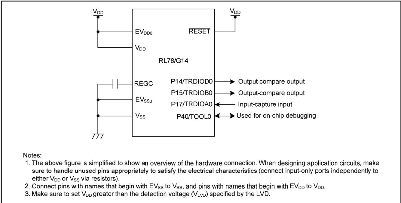
**Figure 3.1 Hardware Configuration**
