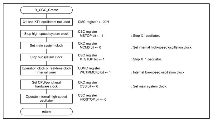
Figure 4.5 Initial Setting of the CPU
