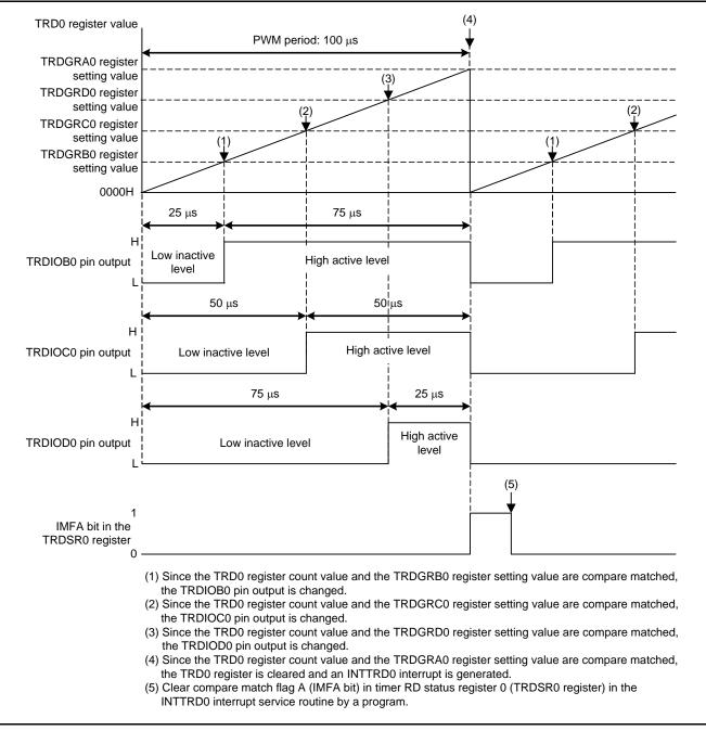
Figure 4.1 PWM Output Waveform
