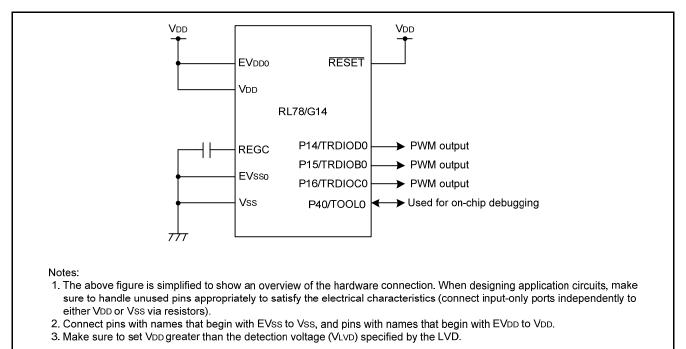
Figure 3.1 Hardware Configuration
