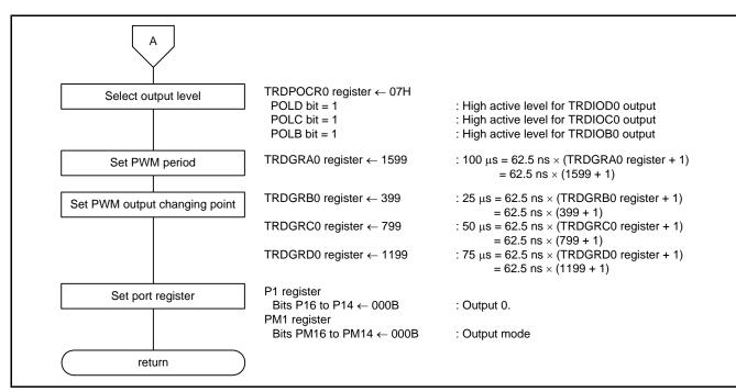
Figure 4.7 Initial Setting of Timer RD (2/2)
